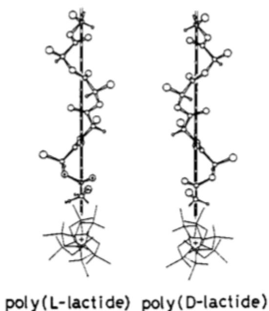
**Figure 20: Chain models of PLLA and PDLA**
