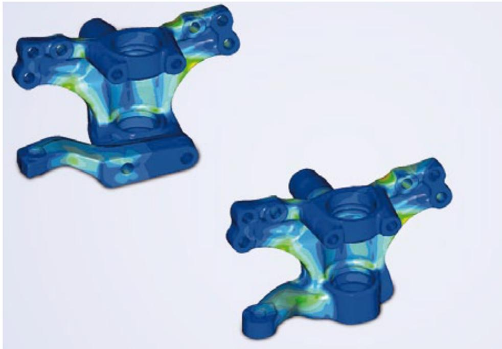
Figure 1.5: FEM Simulation of forged parts [Massivumformung, 2011]
