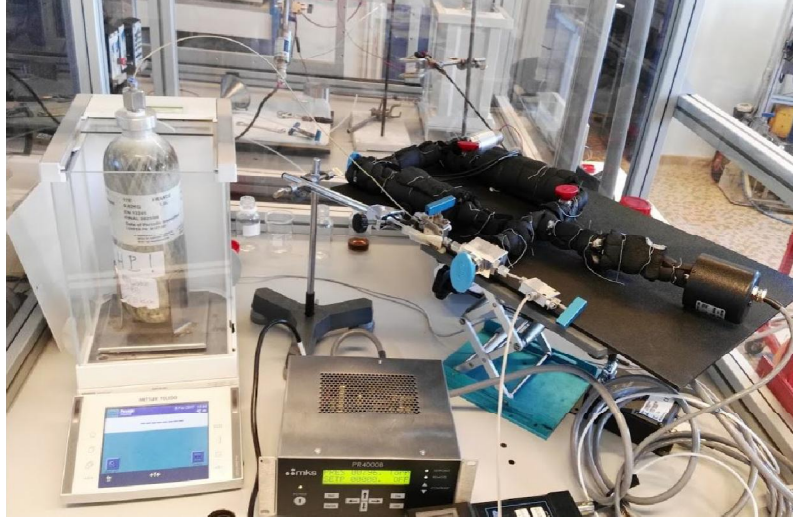
Figure 2.2: Gravimetric volume calibration test
