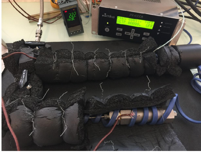
Figure 2.3: Heating system for isothermal conditions of the pure gas adsorption device.
