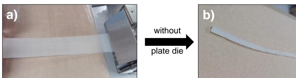
Figure II-6: a) Band-shape extruded samples and b) cylindrical shape of G0_LOW .
