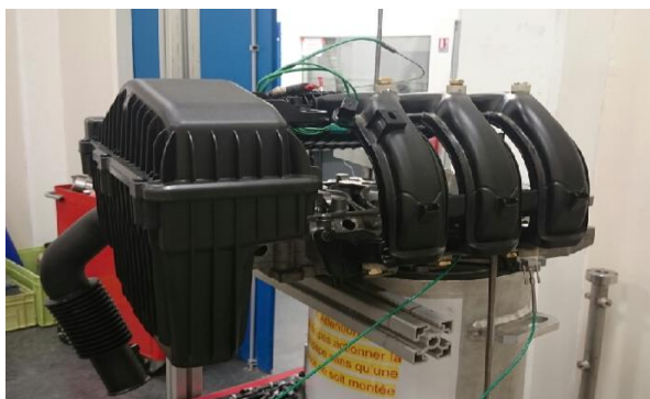
Figure II-19 – DFB tests on EB2 intake system
