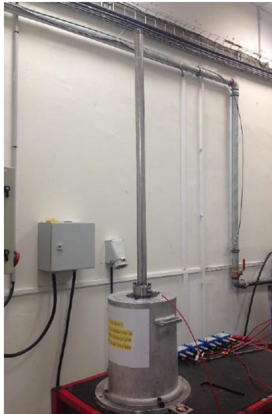
Figure II-11 – Dynamic Flow Bench test using the absolute reference
