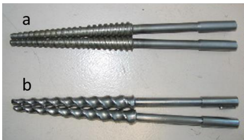
Figure 55 Configuration de vis contra-rotative (a) et co-rotative (b)
