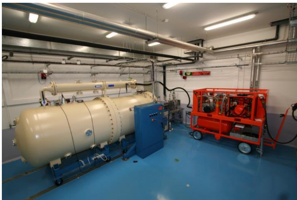
Figure 3.4: Illustration of the Pelletron SIRIUS Van de Graaff electron accelerator
