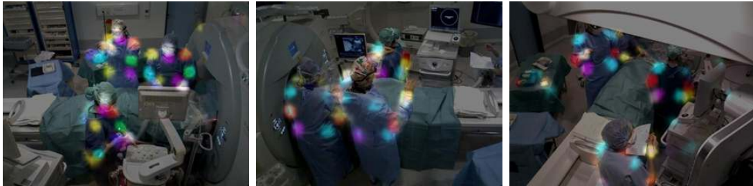
Figure 6.4: Part detection score maps. These score maps are generated using Deep3DPS ( RGB-D ) and overlaid over the corresponding color images
