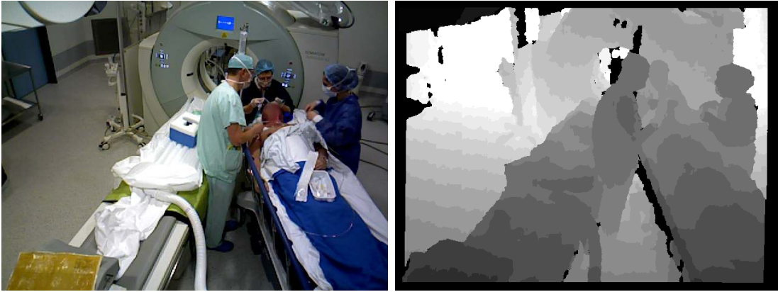
Figure 1.3: A pair of color and depth images captured using an Asus Xtion Pro camera.
