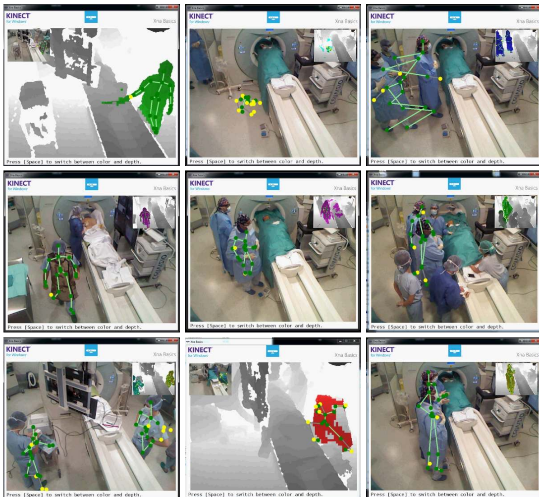
Figure 1.7: Examples of pose estimation results from Kinect skeleton tracker [Shotton 2012]. These frames are extracted from video recordings of the Kinect skeleton tracker evaluated in an operating room. We have extracted the frames after the first hundred frames to make sure that the tracker is initialized. The segmented foregrounds are indicated by different colors on the depth images. The estimated skeletons are overlaid on the color images. (Picture best seen in color)
