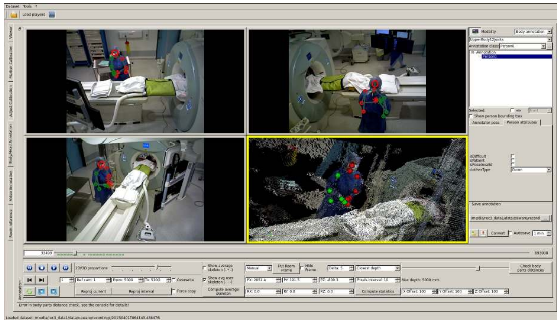
Figure 6.2: Annotation tool. Three views and the 3D point cloud (bottom right) are shown in the window. Right side body parts are indicated in green color. Occluded body parts are denoted by crosses. The annotator can move points in either 2D or 3D. The correctness of an annotated skeleton can be verified using both the 3D point cloud and its reprojection to the views.
