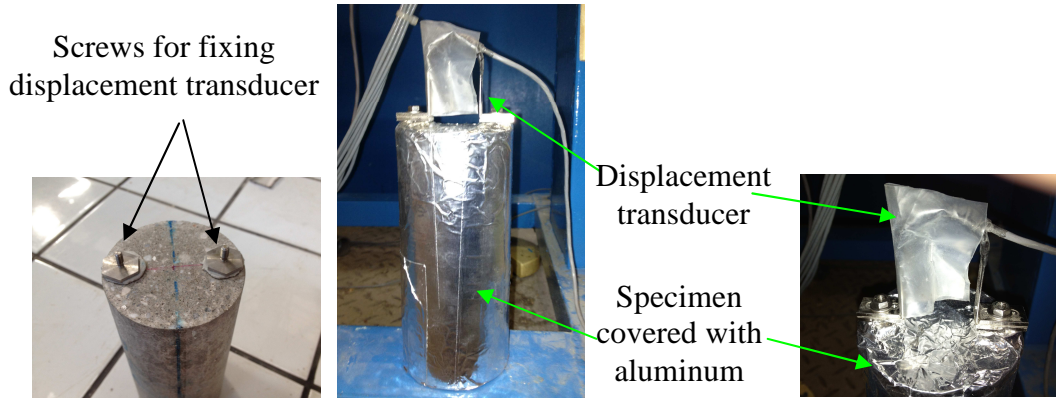
Figure (2.35): Fixing the displacement transducer on a specimen
