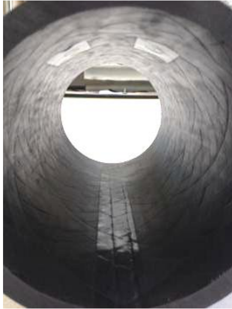
Figure 116 : Groove induced by the two-shell mandrel
