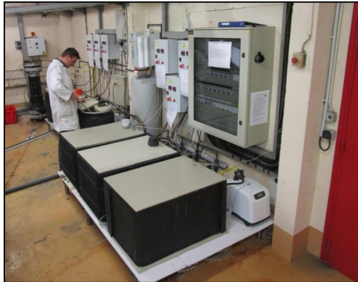
Figure 19 : Sea water aging tanks at Ifremer
