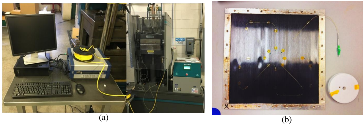
Figure 31 : (a) ODISI Fibre optic sensor and Carver press and (b) Positioning of the fibre optic sensor inside the mould.
