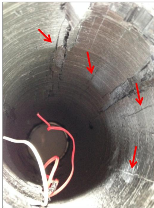
Figure 128 : Kinkbanding failure observed inside the [0/±88] cylinder
