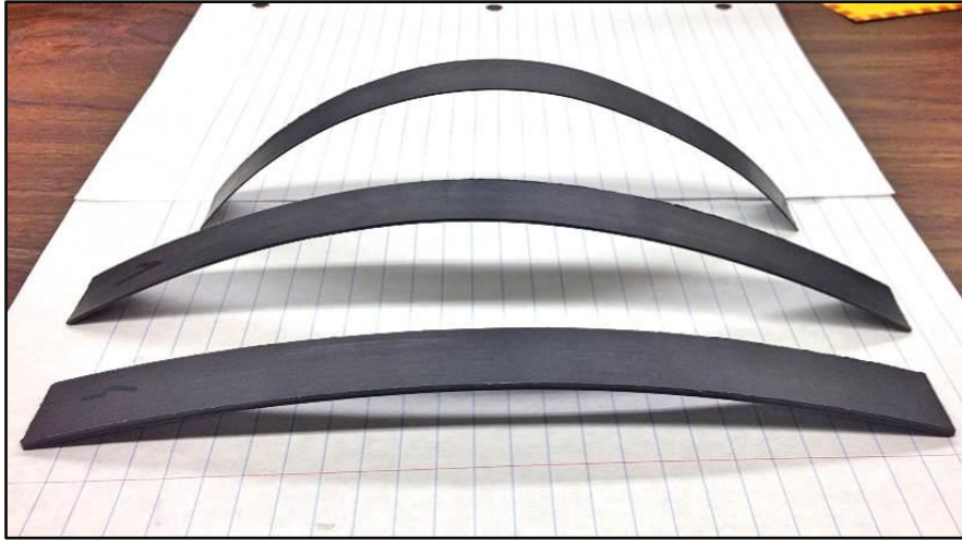
Figure 32 : Asymmetric laminates, from back to front: [0_2/90_2] , [0_4/90_4] and [0_8/90_8]
