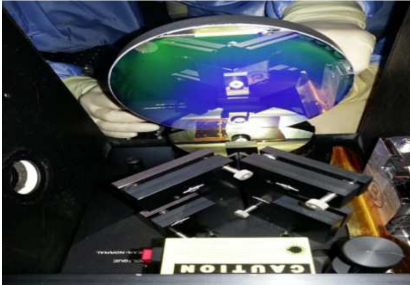
Figure 3.13.: Flight grating being mounted on the Perkin Elmer in its W-mode. Manipulator: R. Grange.
