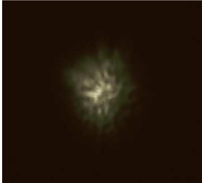
Figure 5.4.: Aberration measured from the Field Corrector (the image is about 9 arcsec on the side).
