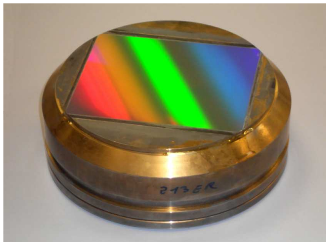
Figure 2.9.: Grating replica on its deformable matrix. Credit: Lemaitre et al., 2014
