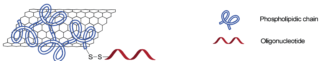
Figure 3.2 Schematic representation of oligonucleotide-S-S-CNT conjugates used in ref. [12] and [13].
