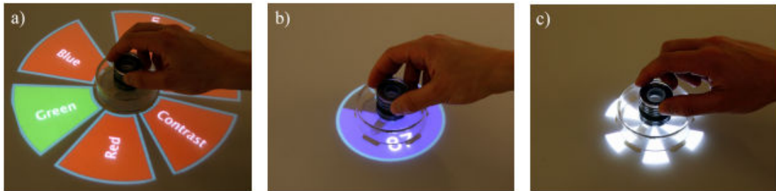
Figure 4: SLAP Knob user interface. a) Selecting image property from menu; b) Setting continuous value; c) Relative navigation for frame stepping in videos (Weiss et al., 2009).
