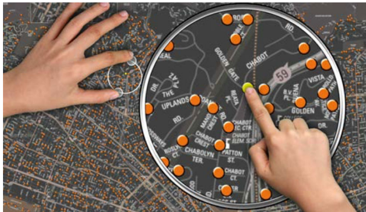
Figure 28: FingerGlass allows using the coarse hand to set a region to magnify and using the fine hand to select objects in the magnified view (Käser et al., 2011).
