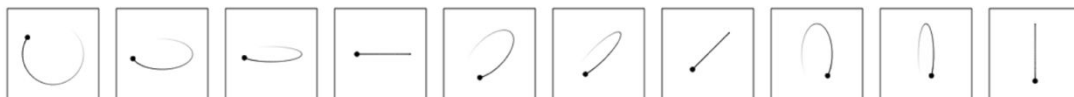
Figure 38: Sample of some of the cyclic elliptical motions used as the basis for the motion-pointing method (Fekete et al., 2009).
