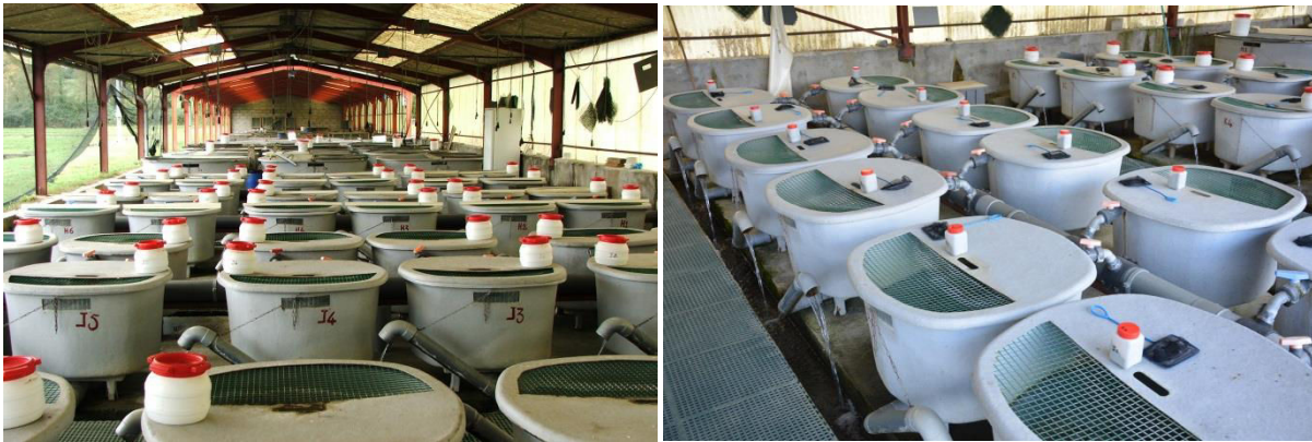
Figure 2. 1 The experimental flow through rearing system setup used for conducting feeding trials at the INRA experimental farm, Donzacq
