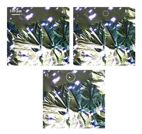
**Figure 5. 5.** Nucleation of a tiny crystal (white circle) at the water drop surface far from a CP droplet (T = 0°C). a)  $t_0$ , b)  $t_0 + <1$ s, c)  $t_0 + 1$ s. DIC imaging mode. Experiment 2014/11/17.
