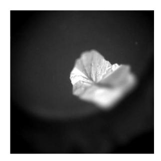
**Figure 2. 22.** Hydrate crystal at the interface water/cyclopentane using the fluorescence imaging mode. DASPI molecules are added to the water with a concentration  $2 \cdot 10^{-6}$  M.
