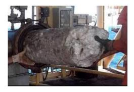
Figure 1. 1. Natural gas hydrates blocking a pipeline due to the cold temperatures and high pressures.
