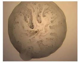
Emulsion moving towards the center  $t_0+3 \text{ min, } T=8^\circ C$
