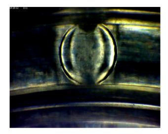
**Figure 4. 9.** Complete dissociation of the hydrate system water + PVCap (100 ppm)/CP at 13°C. See that a liquid/liquid interface is observed.
