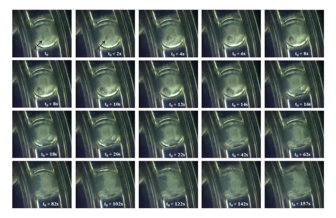
**Figure 3. 10.** Snapshots of (second) hydrate formation in a single water drop (melting conditions of the first hydrate:  $T_{dis} = 8.8$ °C,  $t_{dis} = 2$  h). CP hydrate appears at  $t_0$  (T ~ 2°C) as a darker spot (black arrow) in the emulsion, which then moves slowly and reaches the drop apex at  $t_0 + 17.4$  s; then hydrate grows and covers the whole drop surface within about 2.5 min.
