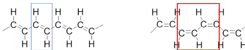
Figure 2.11 Trans -polyacetylene (right) and cis -polyacetylene (left). In the blue and red box are reported the repeat units.
