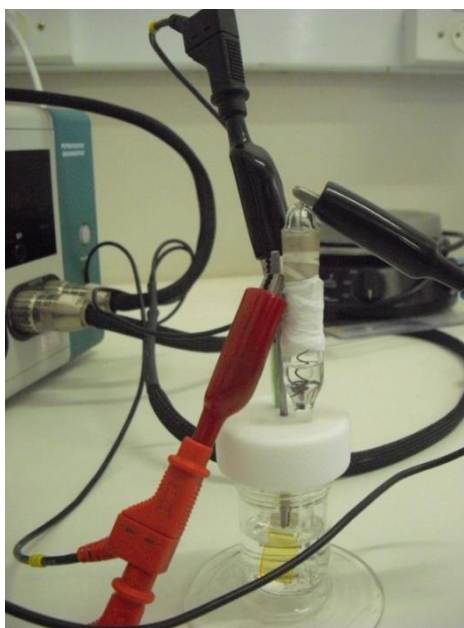
Figure 22: Electrochemical cell and experimental setup for CV measurements.
