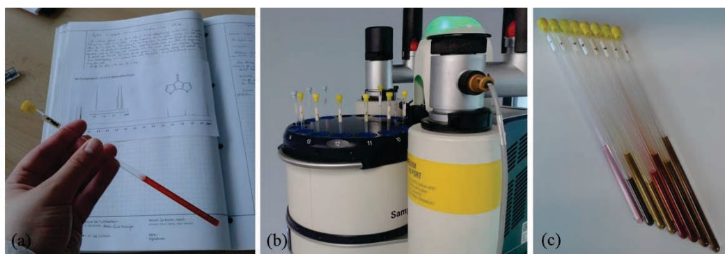
Figure 9: (a) The NMR analysis allows for the deducing of the molecular structure of the compounds obtained at each of the steps of the monomer synthesis route, (b) part of the Bruker UltraShield 400 Magnet NMR instrument and (c) some NMR tubes with different products inside dissolved in \text{CDCl}_3 .
