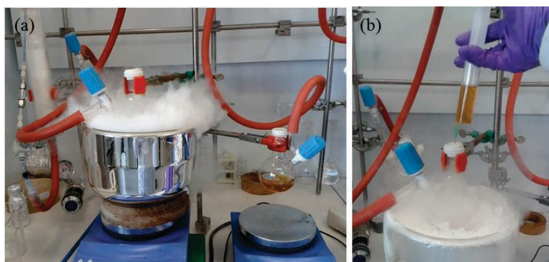
Figure 10: (a) experimental apparatus for chemical reaction using liquid nitrogen and (b) time of dropwise addition of thiophene-3-carboxaldehyde.
