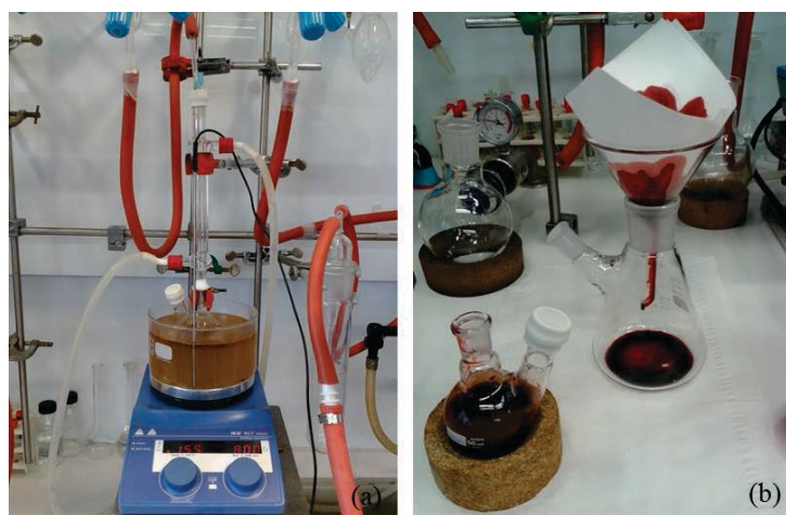
Figure 12: (a) experimental apparatus for the chemical reaction using the reflux system and (b) filtering the remaining Cu after the reaction.
