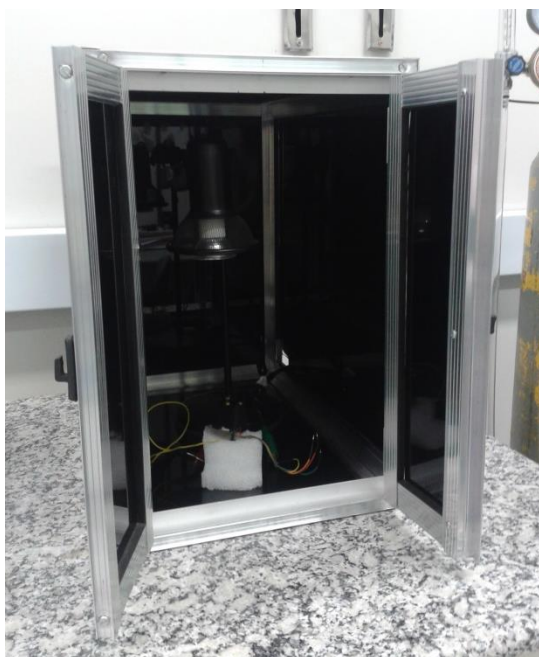
Figure 25: Experimental apparatus used to carry out electrical measurements in dark and under illumination of the halogen lamp of 150 mW/cm 2 power.
