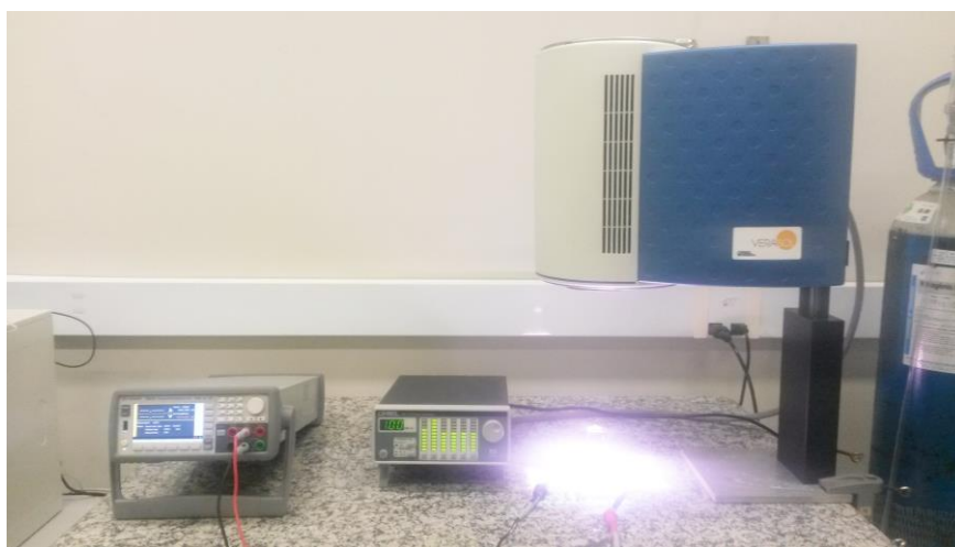
Figure 26: Experimental apparatus used to carry out photovoltaic measurements in dark and under illumination of the Oriel VERASOL solar simulator (100 mW/cm 2 – AM 1.5).
