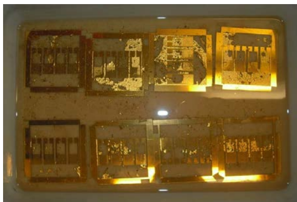
Figure 29: Lift-off step under acetone, to remove the photoresist and metal film, the last process of the fabrication of the IDE.
