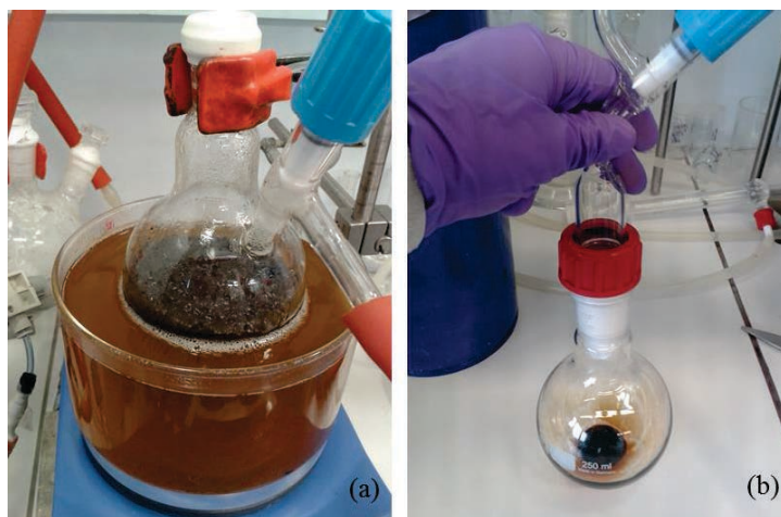
Figure 13: (a) experimental apparatus for the chemical reaction at 180 °C and (b) resulting product left under vacuum after removal of the solvent by the rotary evaporator system.
