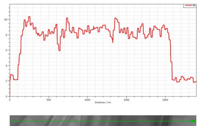
Figure 175 – Mn profiles of 10h sample: at left are presented selected zones and at right – corresponding Mn evolutions as a function of distance.
