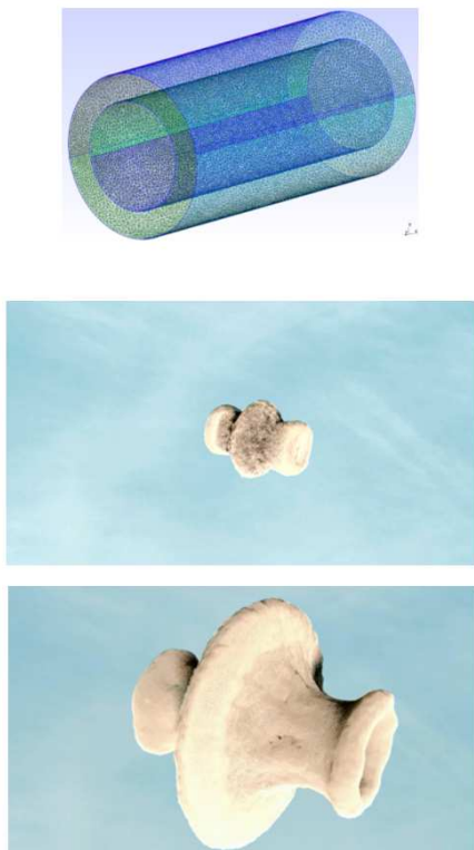
Figure 20: Same explosive charge with liquid layer, first in open air (left view) and second in a bunker, partly opened (right view). The results show liquid water contours at various times.
