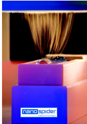
Figure 6: Needleless electrospinning system presented by Elmarco Co.
