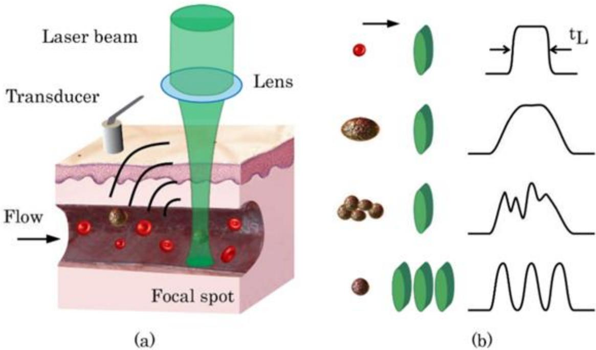
(Color online) (a) PA time-of-flight velocity measurement with cylindrical laser beam. (b) Shapes of PA peaks for different sized objects (illustrated on the left as red or brown circles) and various beam geometries (one- or three-beam; illustrated as green ovals).
