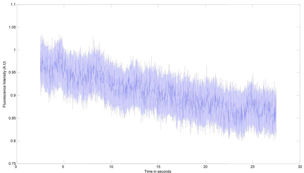
*Figure 32: Representative signal of IVFC experiments. The signal is very noisy, and tends to decrease. Signal processing does not eliminate noise in a sufficient way to identify cell signal. Each time we performed this experiment, we observed the same.*
