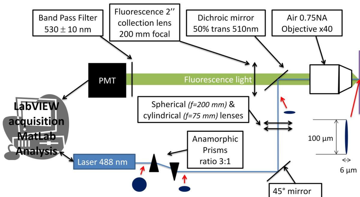
*Figure 26: Experimental set up of IVFC. The laser beam is shaped into a slit by an anamorphic prism duet and by a cylindrical lens. Fluorescence is gathered with a dichroic mirror and with a 2" fluorescence collection lens. A bandpass filter select the light propagating to the detector.*
