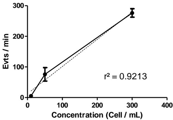
*Figure 30: Link between the number of detected fluorescence events and concentration. The expected linear relation is observed. (Repeated 5 times)*
