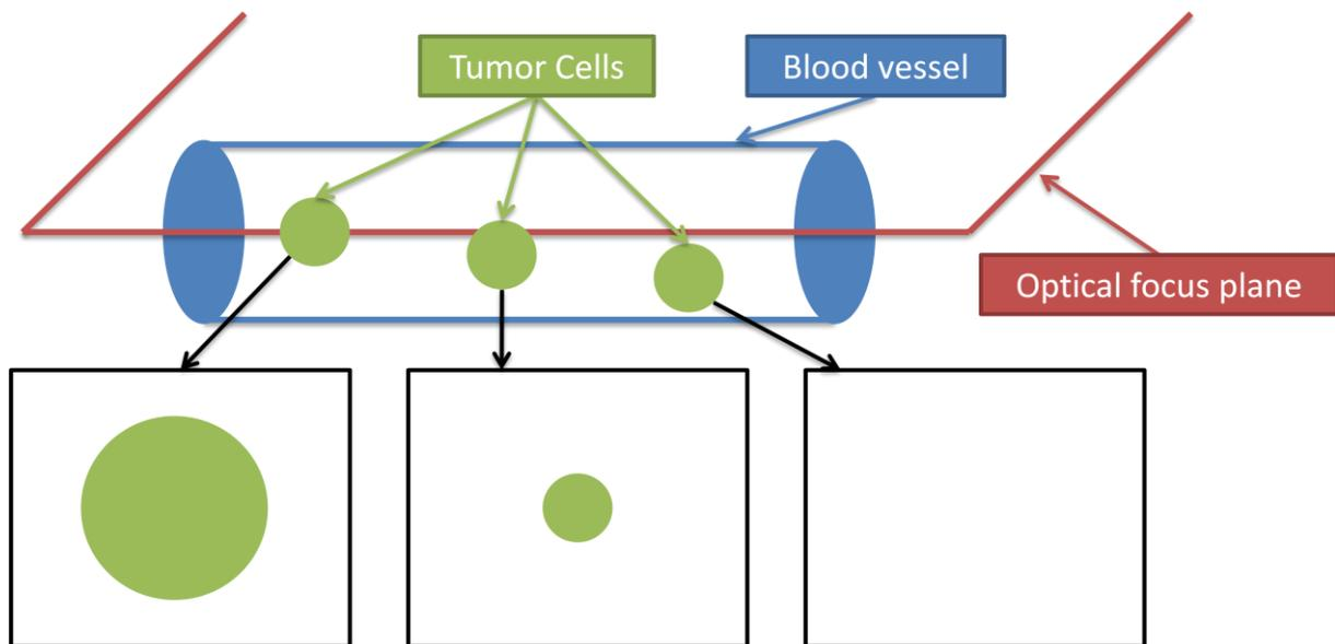
*Figure 25: Scheme showing the problem of confocal microscopy (whether it would be single photons or 2-photons) for the detection of CTCs. The focus plane being thin, the explored volume is very low and the probability to miss cells is too high for accurate counting of CTCs.*
