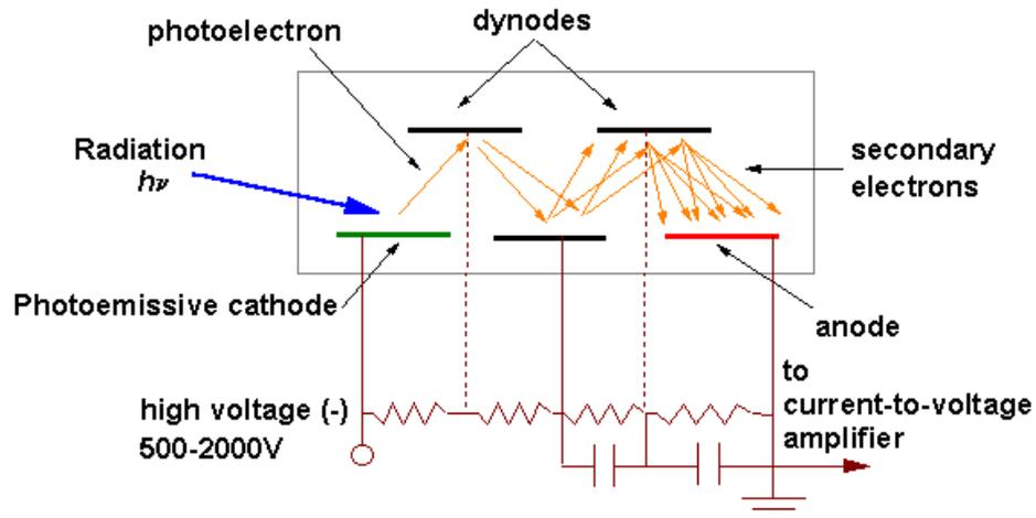
*Figure 27: Scheme of a Photomultiplier Tube. A PMT is very sensitive (photon counting) light sensor.*
