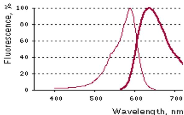
*Figure 7: Absorption and emission spectra of TagFP635 (aka mKate). Normalized excitation (thin line) and emission (thick line) correspond to wavelength suitable with *in vivo* imaging.*
