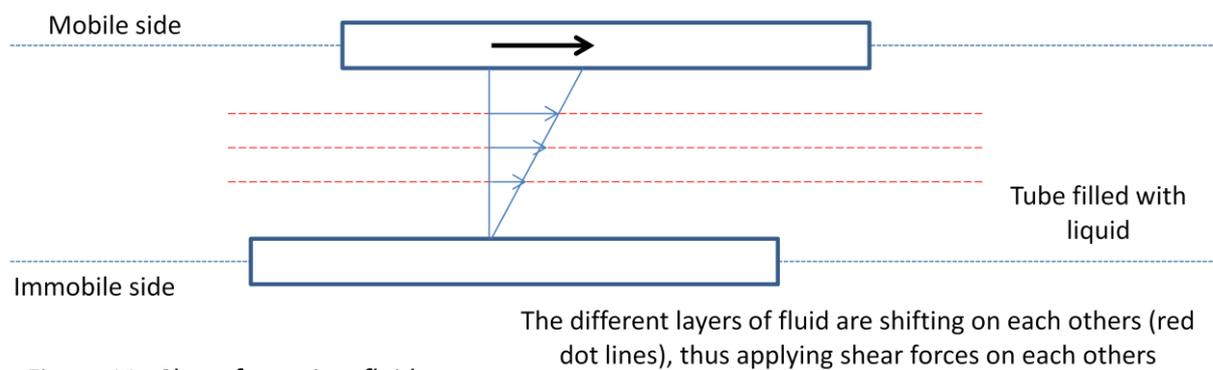
*Figure 11: Shear forces in a fluid.*
