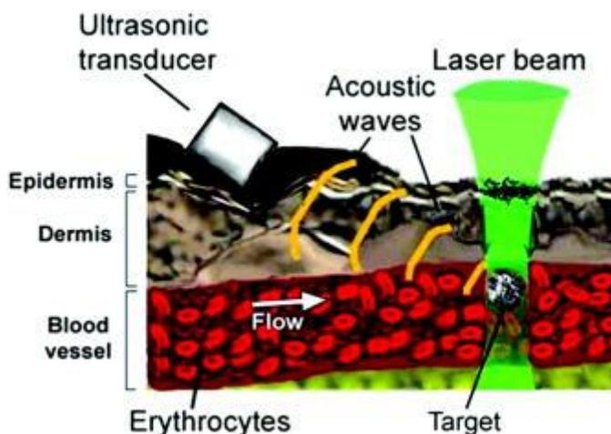
*Figure 9: In vivo Photo Acoustic Cytometry principle. The laser beam warm the flowing cell. The subsequent dilatation of cells produces an acoustic wave that can be detected. From Zharov et al.*
