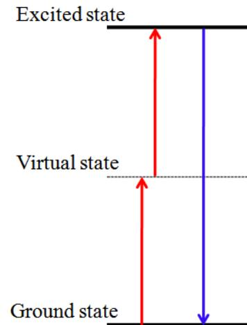
For TPA, the Beer's law (1) becomes a relation (2) that expresses the output intensity as a function of cross section  $\sigma$  (probability that TPA occurs at the molecule level), of concentration  $c$ , and of  $\beta$ , the TPA coefficient. The TPA coefficient may vary according different parameters such as input light frequency, the density of molecules or the incident photon energy.
