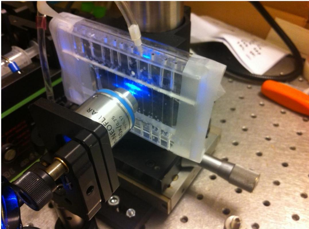
*Figure 29: IVFC in vitro validation. Silicon vessel phantom. 120 $\mu$ m diameter tubes are embedded in a silicon matrix. The slit of light intercepts the vessel phantom and fluorescence of circulating cells is analyzed*
