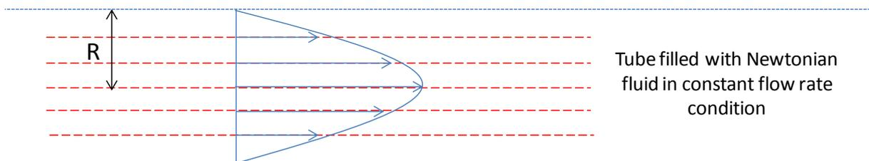
Figure 10: Velocity profile of Poiseuille flow
