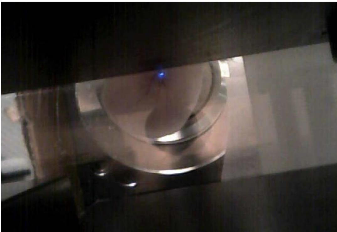
*Figure 31: IVFC laser position monitoring picture. The mouse is anaesthetized with a mix of ketamine / xylazine. Its ear is put between slide and cover slip and the stand his moved until the laser spot is at the correct location. The picture is taken with the monitoring CMOS camera placed*
