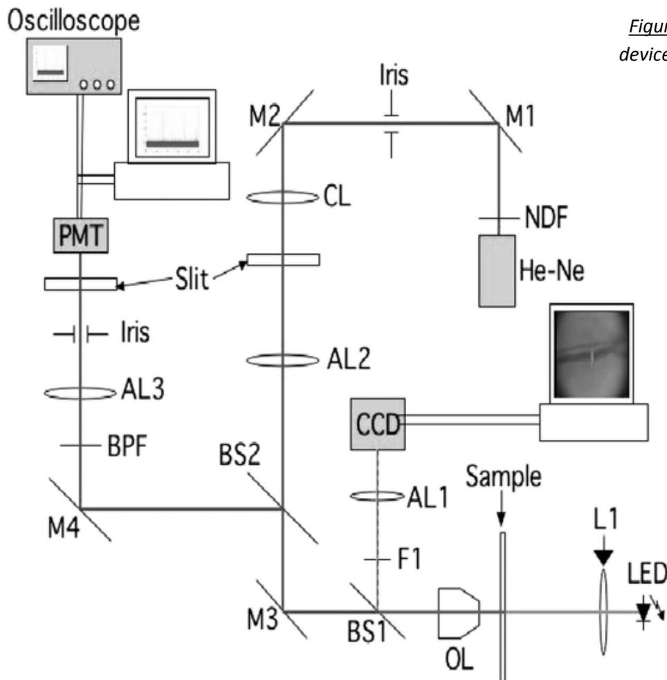
Figure 13 : Experimental IVFC device, from Georgakoudi *et al.*
