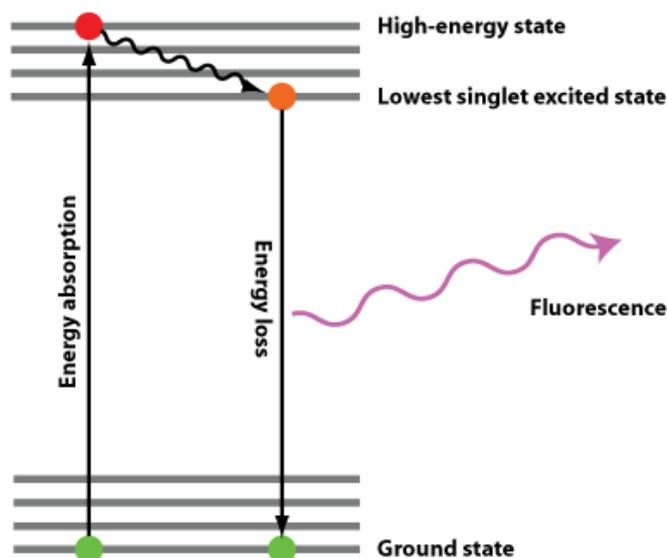
*Figure 5: Energy diagram of a fluorescent molecule excited. Energy is absorbed and allows electrons to access a higher level of energy. A part of this energy is lost in vibration transitions and finally the electrons go back to the fundamental state, emitting a fluorescence photon.*
