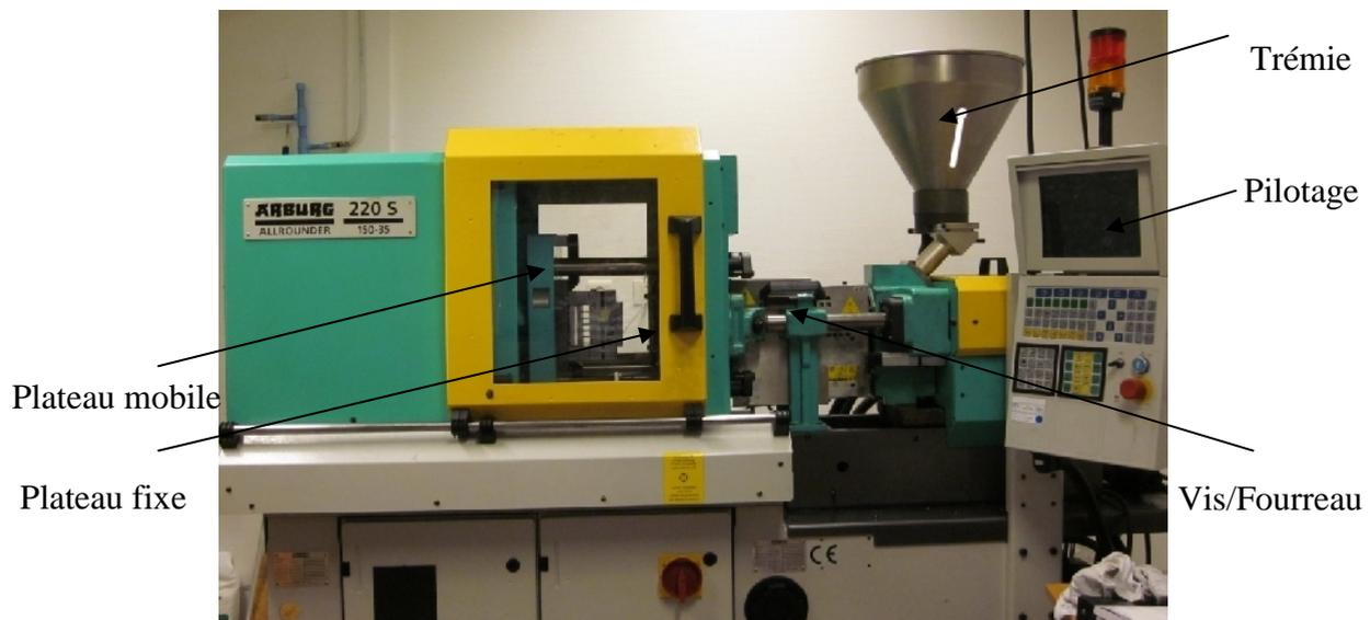
**Figure 2.9** Presse de micro-injection ARBURG Allrounder 220 S
