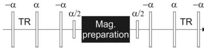
Figure 3.2 – Principle of contrast modification during the steady-state of bSSFP. The steady-state magnetization is stored along the z-direction before magnetization preparation, and is recalled after preparation. Adapted from [Scheffler 2003].
