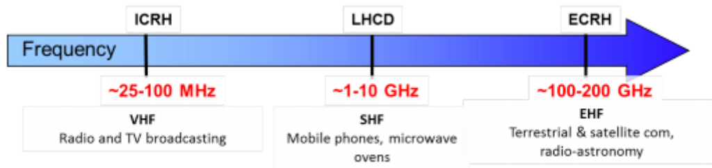
Figure 3.23. Diagram showing the frequency bandwidths used to heat or for current drive in tokamaks.
