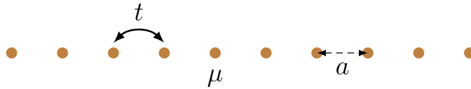
Figure 3.1: One-dimensional tight-binding lattice. \mu is each site chemical potential, a is the lattice constant and t is the nearest neighbor hopping amplitude.
