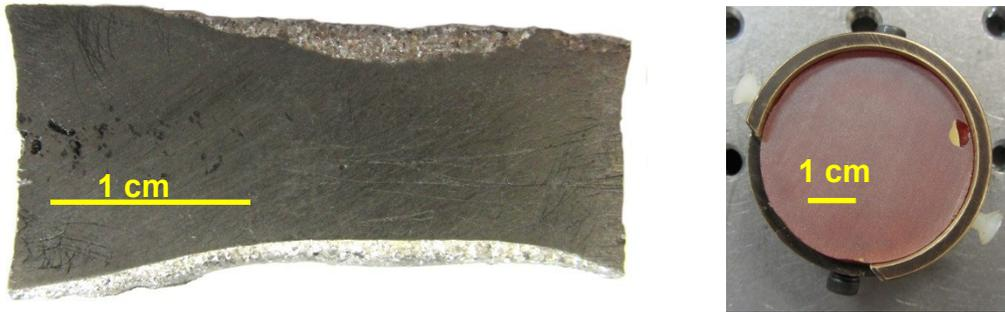
**Figure II.2.** Pictures of typical targets used in the PLD process: GST (left) and GLS (right).
