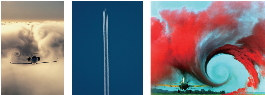
(a) Wake vortices of Learjet 60 in cloud [2] (b) Wake vortices at high altitude as contrail [3] (c) Wake vortices made visible in a NASA test by using colored smoke rising from the ground [4]
