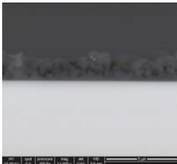
Figure 21. Cross sectional SEM images obtained from the plasma polymers ppAA under conditions corresponding to the Y_{low} values and after 80 passes.
