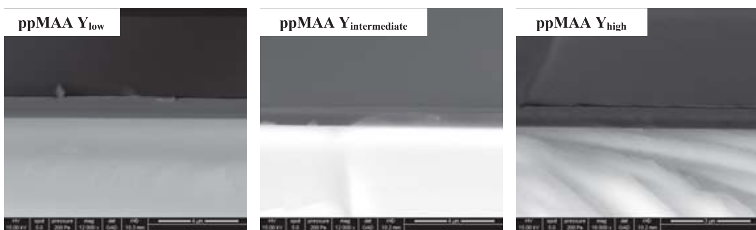
Figure 1. Cross sectional SEM images obtained from the plasma polymers ppAA and ppMAA under different Y conditions and after 80 passes. The scale bars are different in the different micrographs.
