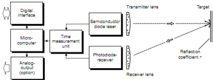
Figure 2.1: Lidar principle of operation (from (67)).
