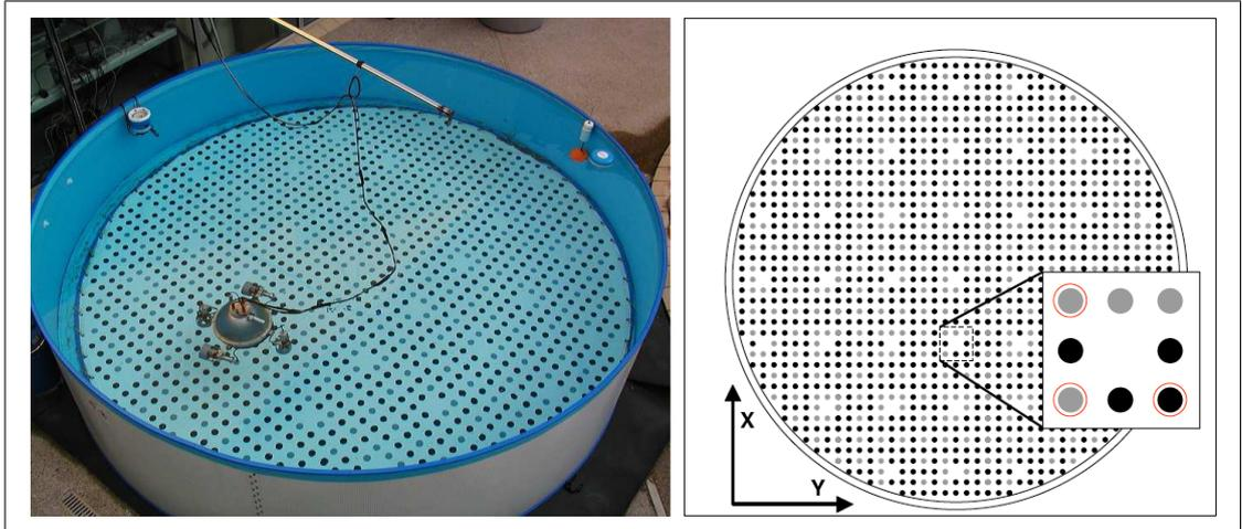
**Figure 4.4:** Localization of the autonomous underwater robot URIS using a pattern coded grid from (8). The robot and its environment (left), and the pattern coded grid (right) where three circles used to determine robot orientation are highlighted by red outlines in the zoomed-in view and the remaining five are used to encode a position on the grid.
