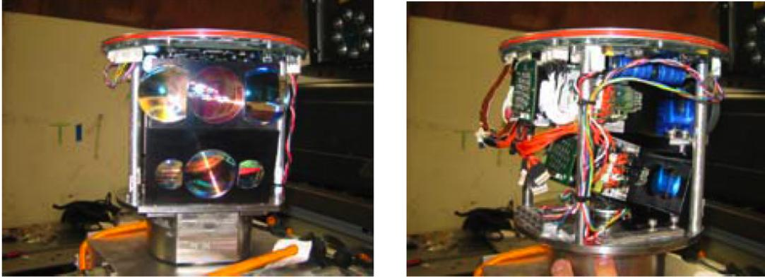
**Figure 2.12:** Velodyne lidar interior from (81): The figure shows four transmitter lenses corresponding to the four laser groups each. For both the upper and the lower block, a receiver lens is located between the transmitter lenses of right and left laser group of the corresponding block.
