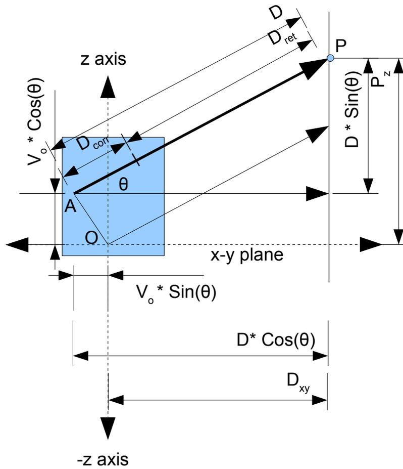
Figure 3.1: Side view of the lidar.
