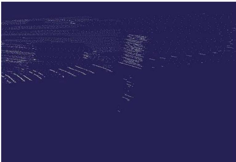
**Figure 2.17:** Phantom points because of very high reflectivity targets (from (71))
