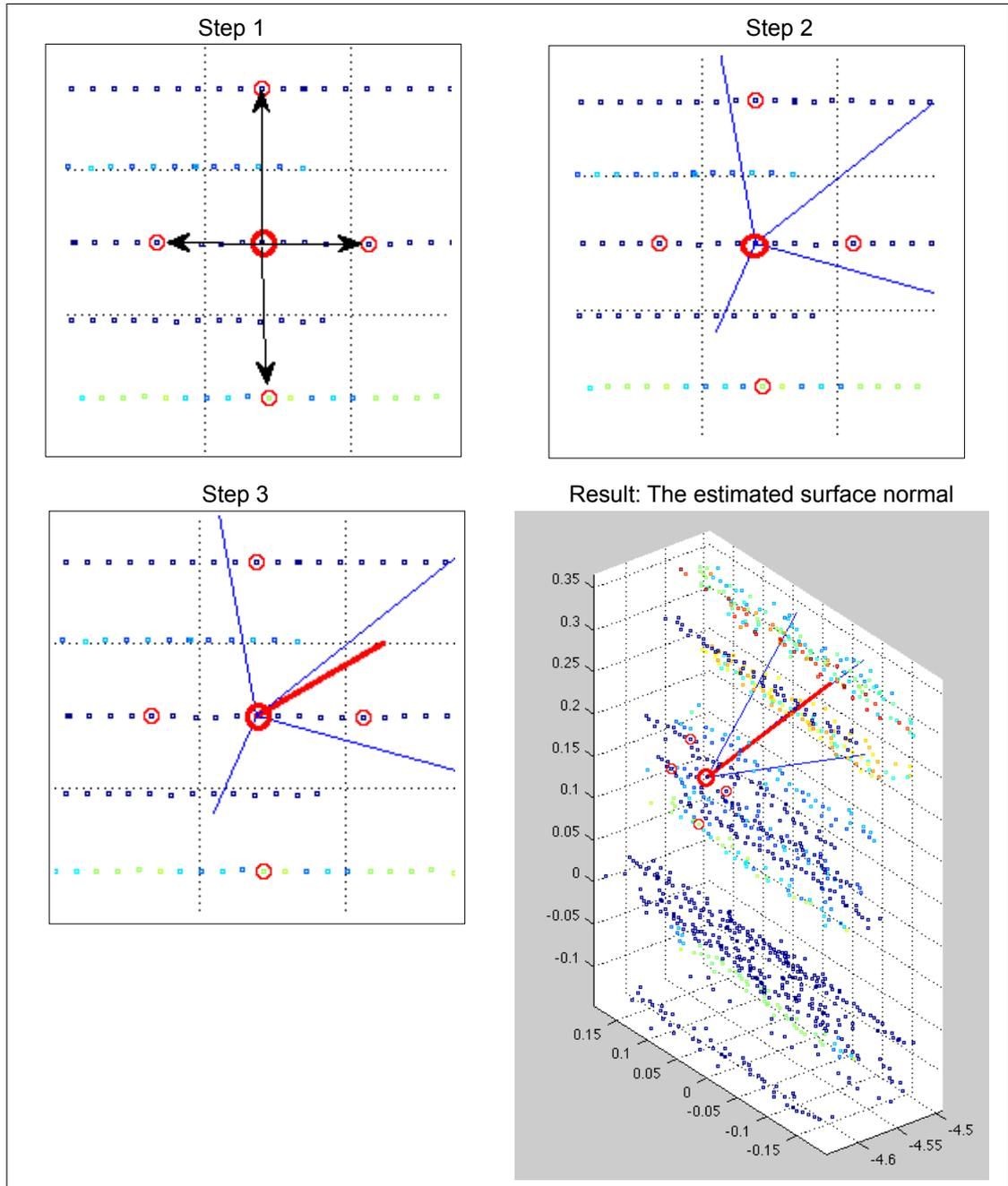
**Figure 5.5:** Surface normal estimation by exploiting Velodyne laser beam arrangement: Four neighbors and the corresponding vectors (top-left), the four cross products shown as blue lines (top-right), geometrical average of the four cross products shown as the red line is the estimated surface normal (bottom-left), and the result shown in 3D (bottom-right).
