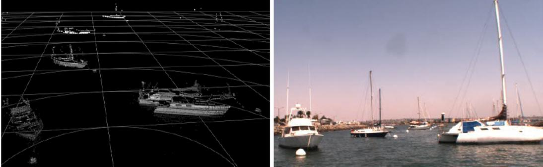
**Figure 2.23:** Maritime data acquisition using HDL-64E (from (28))
