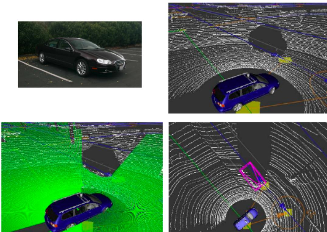
**Figure 2.22:** Tracking of black objects: a black vehicle (top-left), very few laser returns (top-right), virtual scan after black object detection (bottom-left), tracking of detected vehicle (bottom-right) (from (81)).
