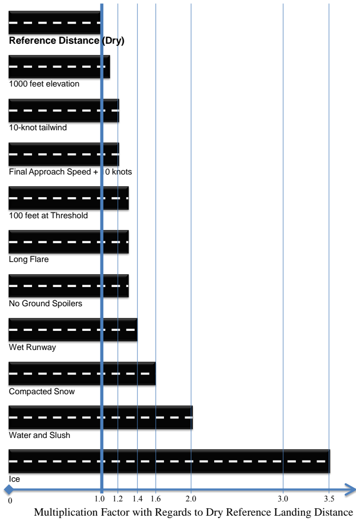
Figure 1.1: Factors that can affect the landing distance (Redrawn from [2])
