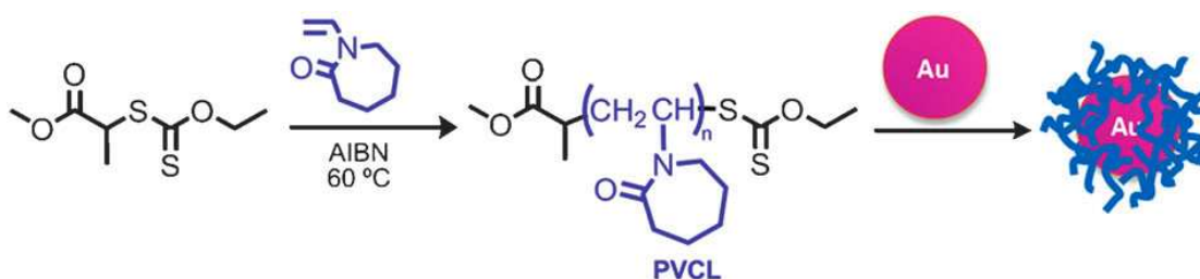
Figure 9. Synthesis of PVCL and coating of AuNPs. Reprinted with permission from ref 202(Marty's group). Copyright 2011 Royal Chemical Society.
