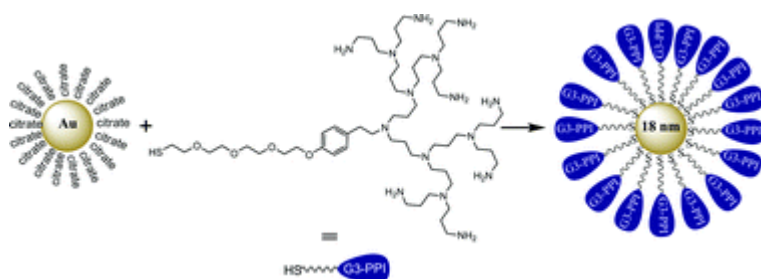
Figure 5. The synthetic routes for the thiol-dendron-stabilized AuNPs. Reprinted with permission from ref 113 (Daniel's group). Copyright 2011 Royal Society of Chemistry.
