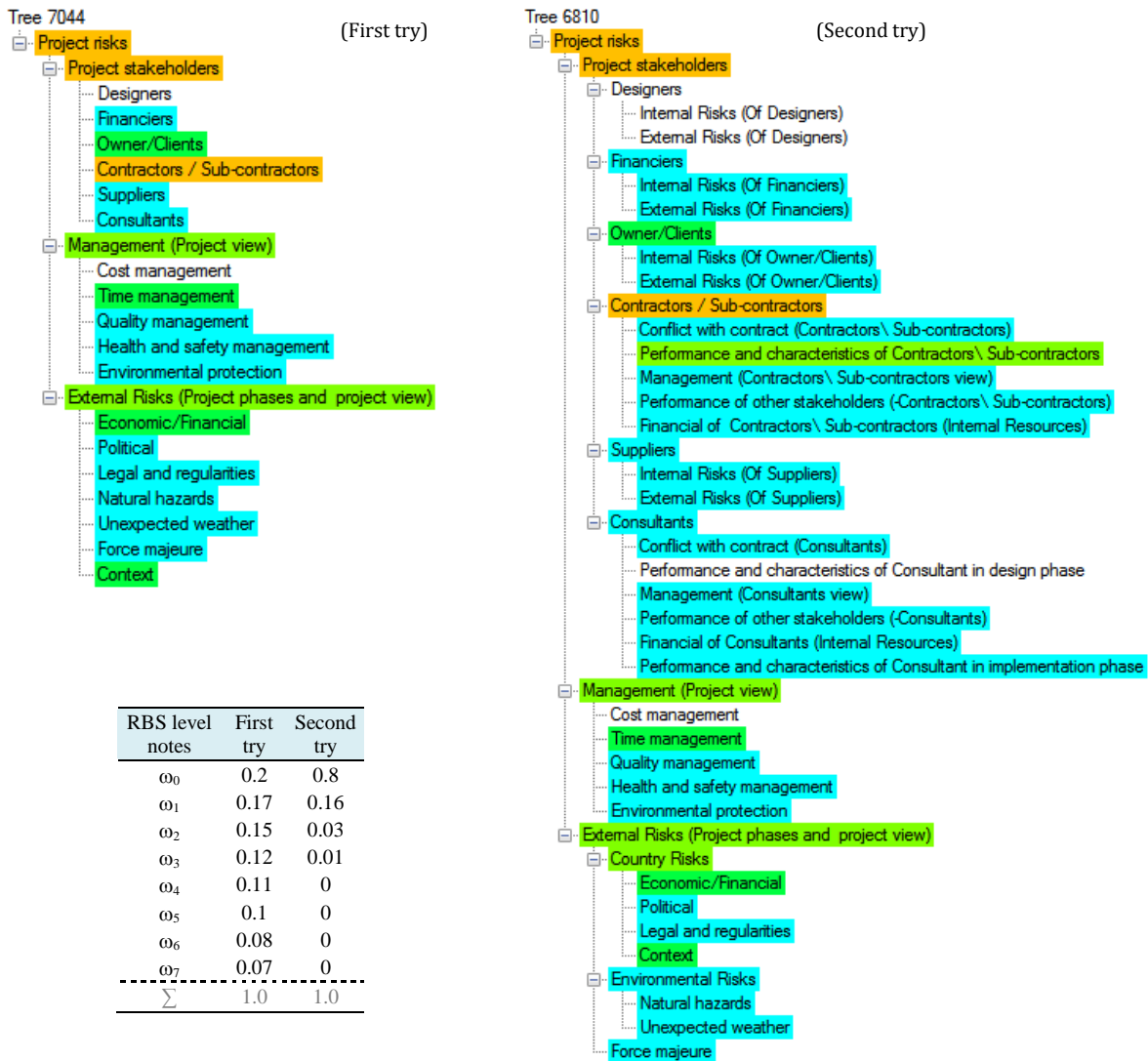
Figure 4-40. Effect of the RBS level notes ( \omega_i ) on tailored RBS generation
