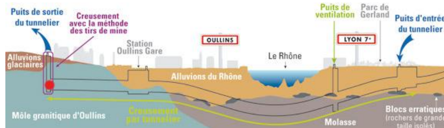
Figure 4-12. TBM arrival to the exit shaft
