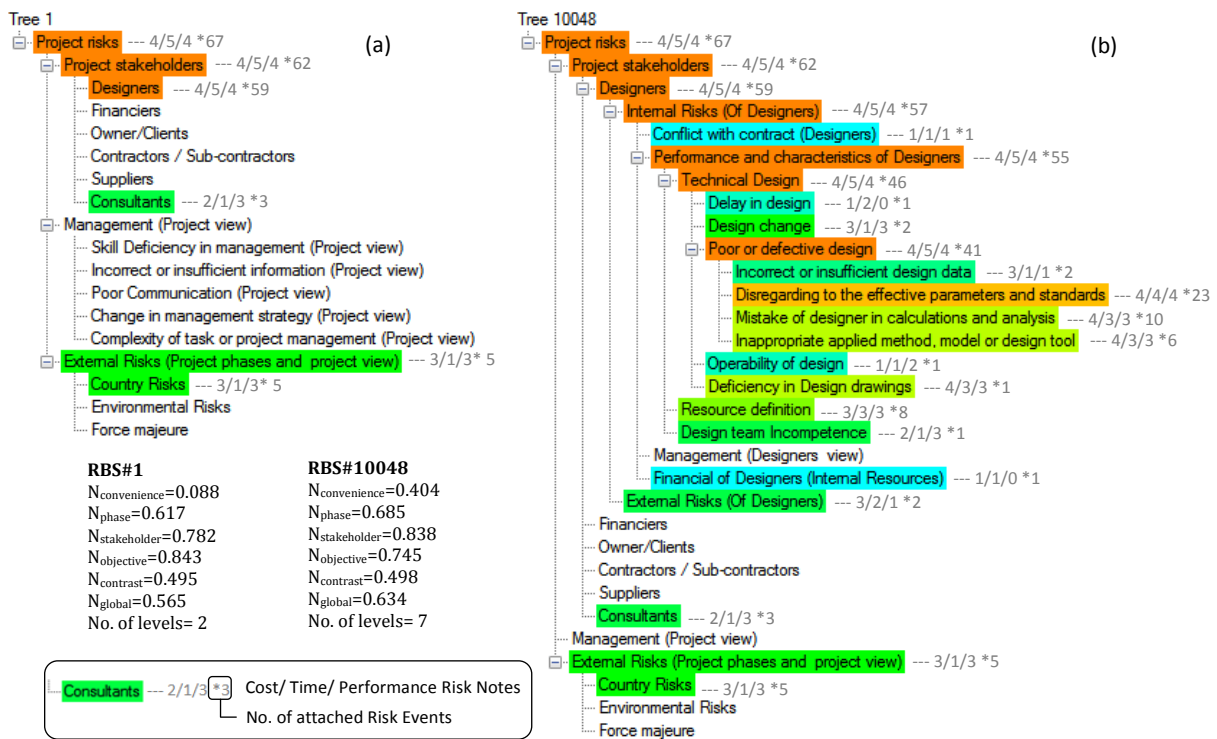
Figure 4-33. a) Tailored RBS for the project designers b) Focus on risks related to designers
