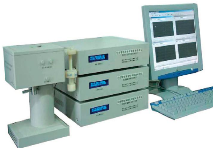
Figure 14. MPI-A capillary electrophoresis-electrogenerated chemiluminescent analyser developed at the Changchun Institute of Applied Chemistry, Chinese Academy of Sciences, and manufactured by Xi'an Remax Electronic Co. Ltd. 1
