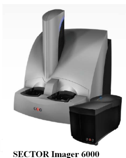
Figure 18. Commercial ECL imager from Meso Scale Discovery. The instrument use ultra-low noise CCD camera and it is suitable for single and multiplexed assay formats. 7
