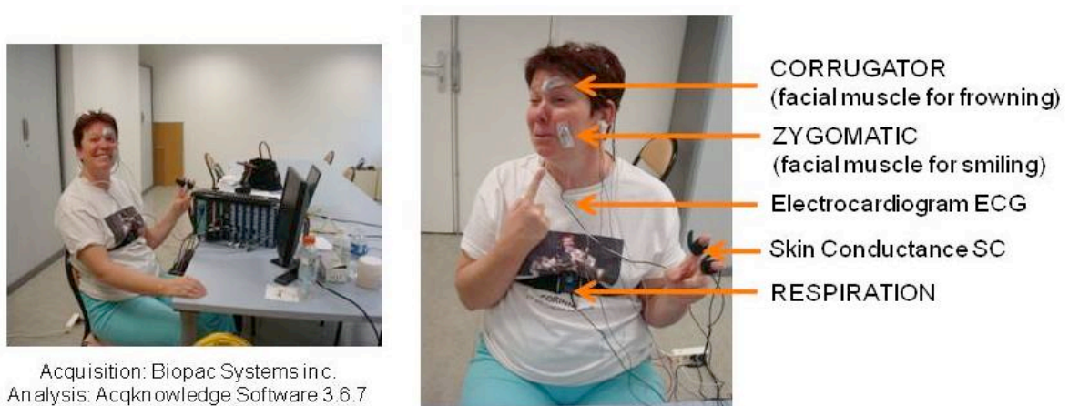
Fig. 7. Illustration of the electrodes placement for the physiological acquisitions
