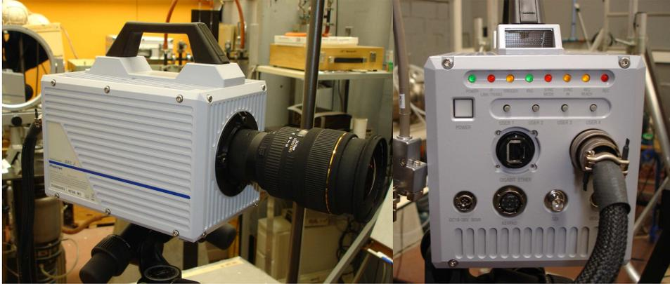
FIGURE 2.3 – Caméra ultra-rapide PHOTRON FASTCAM SA 1.1.
