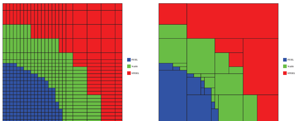
Figure 3.11: 2D conforming (left) and non conforming (right) mesh
