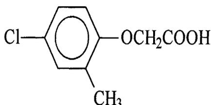
**Figure 11:** Chemical structure of MCPA
