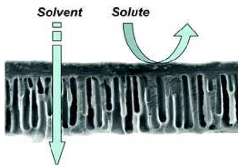
**Figure 45.** Solvent-resistant nanofiltration: separating on a molecular level. Reprinted with permission of the Royal Society of Chemistry (ref. 873, Vankelekom's group).
