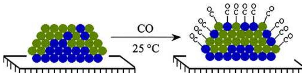
**Figure 44.** Bimetallic dendrimer-stabilized nanoparticles (DSNs) used to prepare supported Pt–Au catalysts within the bulk miscibility gap for a binary system. Reprinted with permission of the American Chemical Society (ref. 861, Chandler's group).
