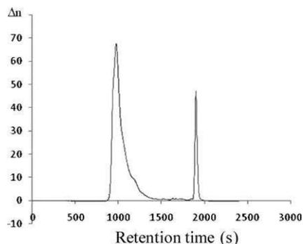
**Fig. 1** Size exclusion chromatogram (SEC) of **5** (left) using polystyrene as the reference and 1,3,5-trichlorobenzene as a marker (shown on the right). The SEC was carried out using a refractometer.  $\Delta n$  is the variation of the refractive index as a function of time (seconds).
