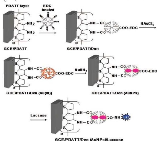
**Figure 109.** Schematic representation of the fabrication of PDATT/Den(AuNPs)/laccase-modified electrode. Reprinted with permission of the American Chemical Society (ref. 1688, Shim's group).
