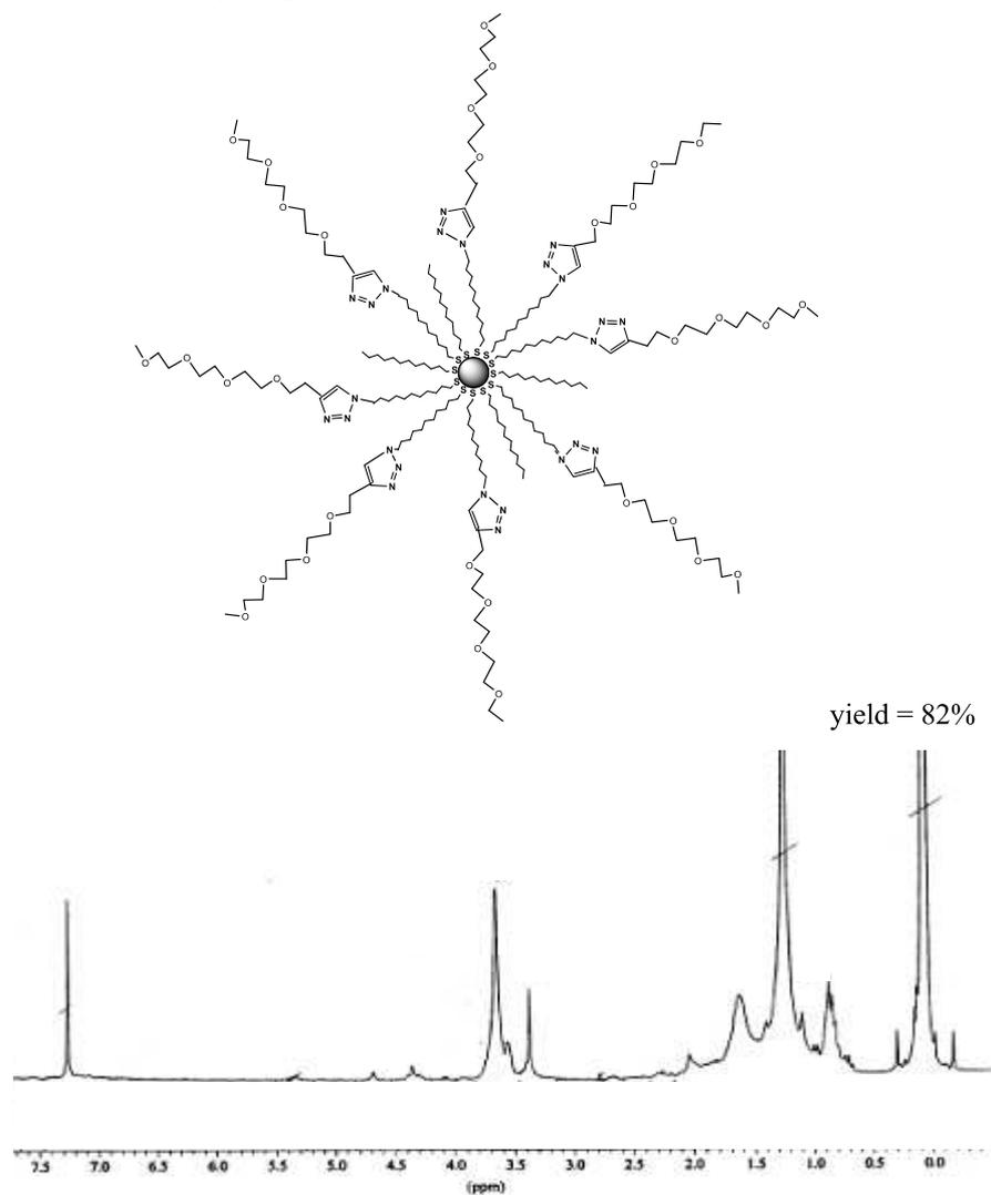
Fig. S15:  $^1\text{H}$  NMR spectrum of AuNPs with tetraethyleneglycol termini in  $\text{CDCl}_3$  ( $\delta$  ppm)
