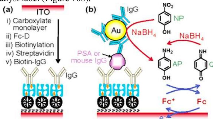
**Figure 108.** (a) Schematic representation of the preparation of an immunosensing layer. (b) Schematic view of electrochemical detection of mouse IgG or PSA. Reprinted with permission of the American Chemical Society (ref. 1676, Yang's group).
