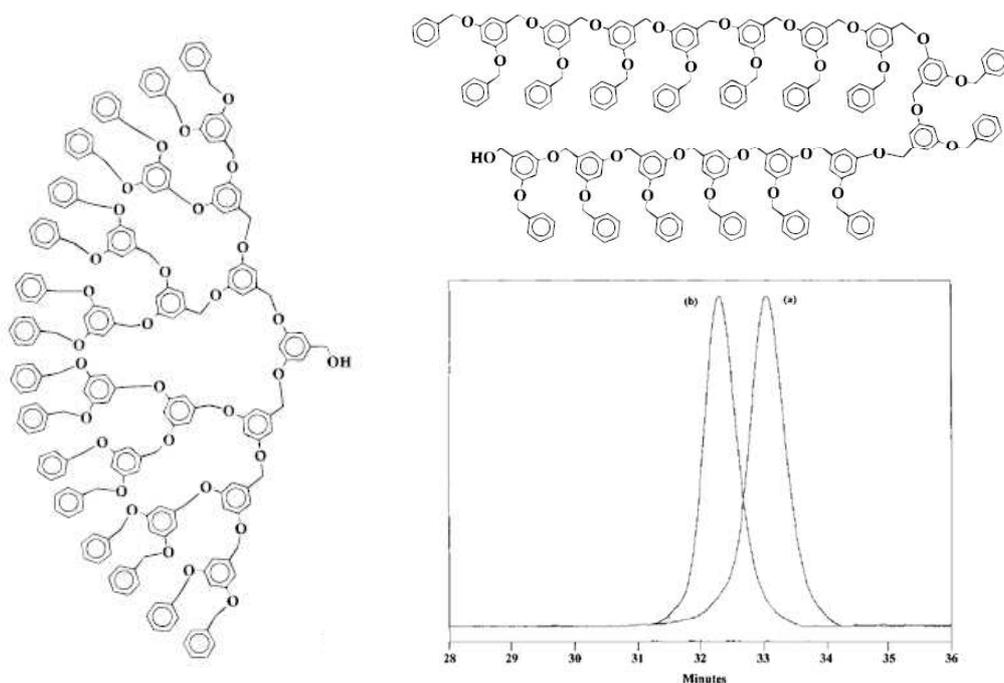
**Figure 4.** Comparative structures of the fourth-generation dendritic alcohol and its exact linear analogue; GPC traces for the (a) fifth generation dendritic alcohol, and (b) the corresponding exact linear analogue. Reprinted with permission of the American Chemical Society (ref. 97, Hawker's group).
