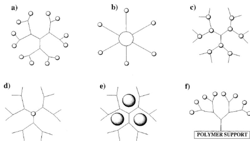
**Figure 41** Various metallodendritic assemblies efficient for metallodendritic catalysis: a) Reetz: Heck reaction 1st recycle in 1997; b) Redox catalysts kinetics shows no steric congestion; c) Kakkar's phosphine-Rh at focal points; d) Van Leeuwen ferrocenyldiphos Pd-centered; e) Crooks: PAMAM inserted Pd nanoparticles; f) Alper's Pd-phosphine dendrons anchored on polystyrene. Reprinted with permission of the American Chemical Society (ref. 799, Astruc's group).
