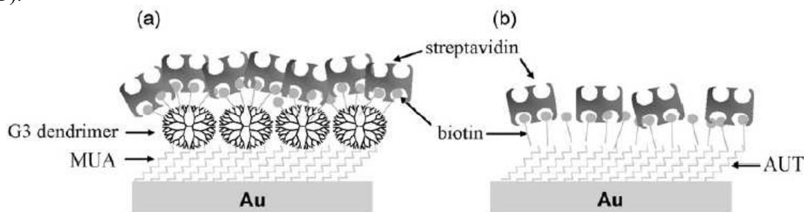
**Figure 23.** Schematic of streptavidin immobilized on a (a) G<sub>3</sub> PAMAM dendrimer monolayer and (b) self-assembled monolayer of 11-amino-1-undecanethiol (AUT) onto gold. Reprinted with permission of Elsevier (ref. 474, Lee's group).
