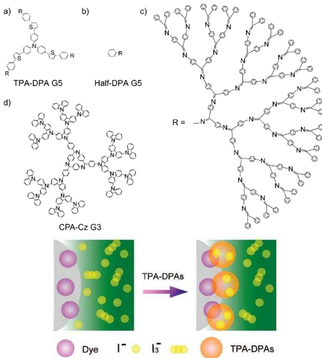
**Figure 17.** Structure of the dendrimers. (a) Triphenylamine core (TPA-DPA  $G_5$ ). (b) Half-dendritic phenylazomethine core (Half-DPA  $G_5$ ). (c) Generation 5 of DPA dendron units. (d) Carbazole dendrimer containing cyclic phenylazomethine of generation 3 (CPA-Cz  $G_3$ ); interface modification by dendrimers on  $\text{TiO}_2$  electrode. Reprinted with permission of the American Chemical Society (ref. 349, Yamamoto's group).
