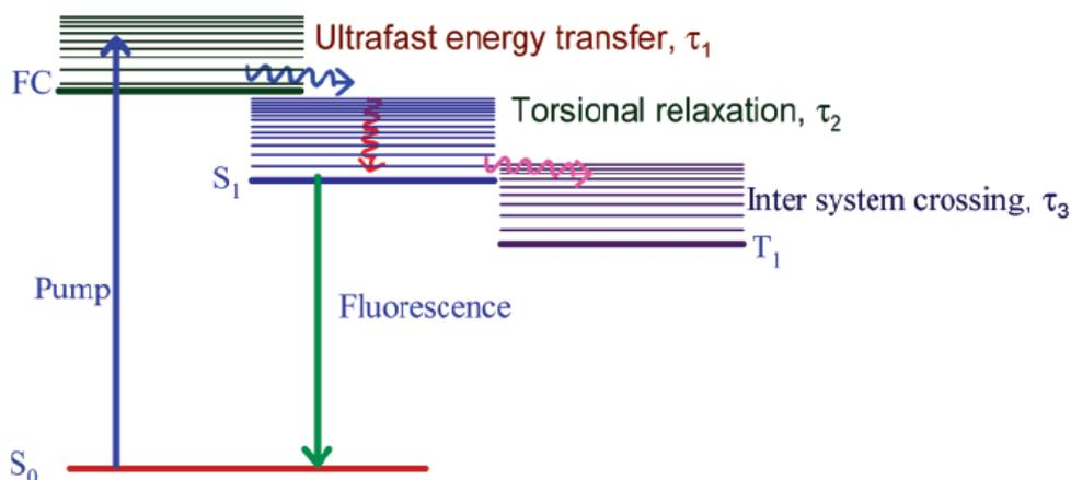
**Figure 18.** Mechanism of excited state deactivation of higher generation thiophene dendrimers. Reprinted with permission of the American Chemical Society (ref. 379, Goodson III's group).
