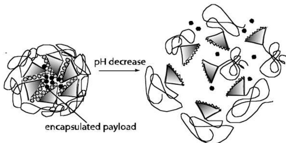
**Figure 75.** Schematic representation of release of guest molecules from a *pH* sensitive micelle of linear-dendritic copolymer. Reprinted with permission of the National Institutes of Health (ref. 1189, Thayumanavan’s group).
