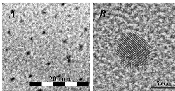
Figure 10. a) TEM of the dendrimer **5** + 1 equiv. of  $\text{HAuCl}_4$  reduced by  $[\text{Fe}^{\text{I}}\text{Cp}(\eta^6\text{-C}_6\text{Me}_6)]$ ; b) HRTEM of the dendrimer **5** + 1 equiv. of  $\text{HAuCl}_4$  reduced by  $[\text{Fe}^{\text{I}}\text{Cp}(\eta^6\text{-C}_6\text{Me}_6)]$ .
