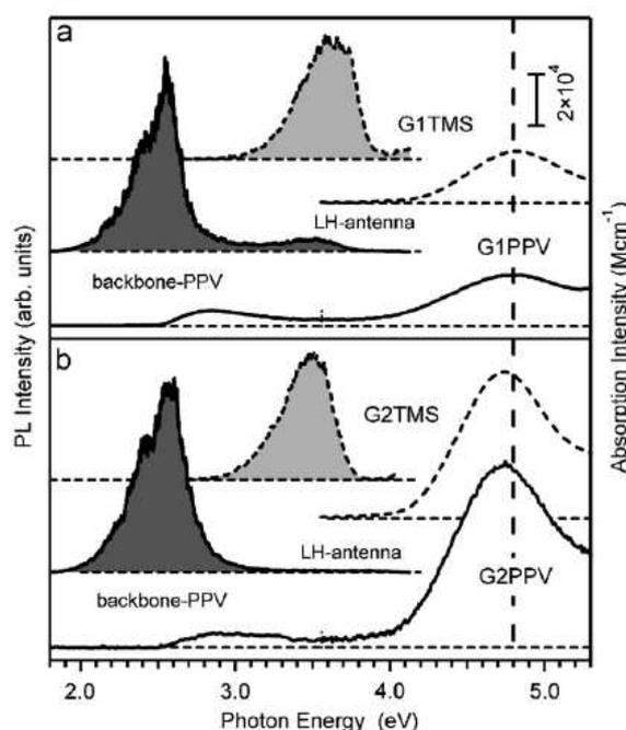
**Figure 15.** Absorption and PL spectra of  $G_n$ PPVs ( $G_n$ PPV:  $n^{\text{th}}$  generation dendrimer with poly(phenylenevinylene) backbone;  $n = 1, 2$ ) and  $G_n$ TMSs ( $G_n$ PPV:  $n^{\text{th}}$  generation dendrimer with trimethylsilyl group backbone;  $n = 1, 2$ ) in solutions. PL spectra are displayed with grayish shadow. Vertical broken line marks the energy of the excitation. Reprinted with permission of Elsevier (ref. 328, Akai's group).
