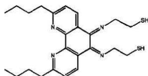
**Fig. 9** Chemical structure of the modified 1,10-phenanthroline ligand that binds to gold nanoparticles through the thiols, and to lithium ion through the chelating phenanthroline nitrogens. Two ligands are required to bind to one lithium ion in a tetrahedral fashion. Reprinted with permission of the Royal Society of Chemistry (ref. 26, Murphy's group).
