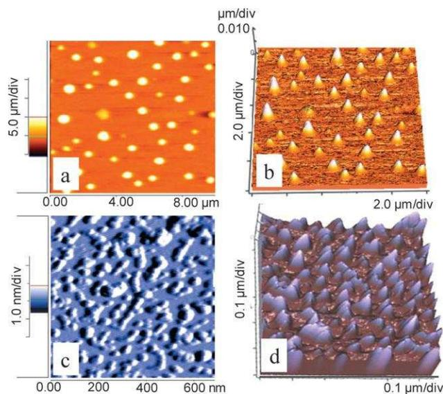
**Fig. 4** AFM image of **5** and **10** on mica surface. (a) Topographic 2D AFM image of **5**. (b) Topographic 3D AFM image of **5**. (c) Amplitude mode 2D AFM image of **10**. (d) Topographic mode 3D AFM image of **10**.
