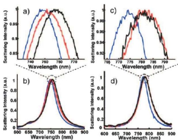
**Fig. 11** (a and b) Scattering spectra of a single gold nanorod after sequential incubation in EG3SH/MHA (blue), biotin (red), and 10 nM streptavidin (black). (c and d) Scattering spectra of a single gold nanorod in EG3SH/MHA (blue), biotin (red), and 100 nM streptavidin presaturated with free biotin (black). Reprinted with permission of the American Chemical Society (ref. 70, Chilkoti's group).
