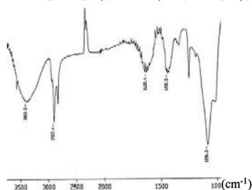
Fig. S16: IR spectrum of AuNPs with tetraethyleneglycol termini
