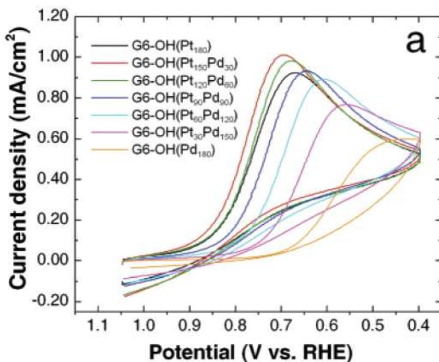
**Figure 59.** Cyclic voltammograms of G<sub>6</sub>-OH(Pt<sub>n</sub>Pd<sub>180-n</sub>)(n = 180, 150, 120, 90, 60, 30, and 0). Reprinted with permission of the American Chemical Society (ref. 1036, Crooks's group).
