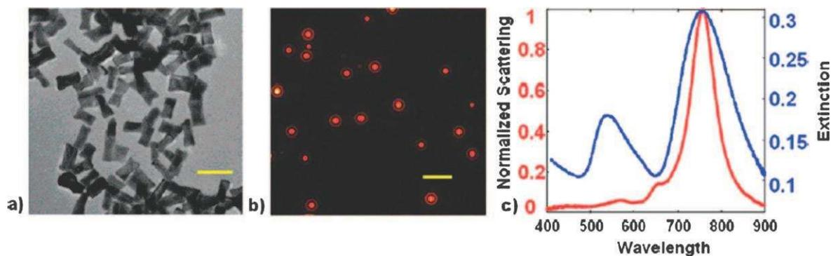
**Fig. 10** (a) TEM of gold nanorods used for biodetection experiments and (b) dark-field micrograph of gold nanorods immobilized on a glass substrate. (c) Scattering spectra of a single gold nanorod on a glass substrate (red) and the extinction spectrum of an ensemble of gold nanorods suspended in water (blue). Scale bar is 100 nm in (a) and 5  $\mu\text{m}$  in (b). Reprinted with permission of the American Chemical Society (ref. 70, Chilkoti's group).
