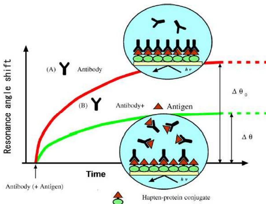
**Figure 22.** Principle of competitive inhibition assay on SPR immunosensor. Reprinted with permission of Elsevier (ref. 464, Singh's group).
