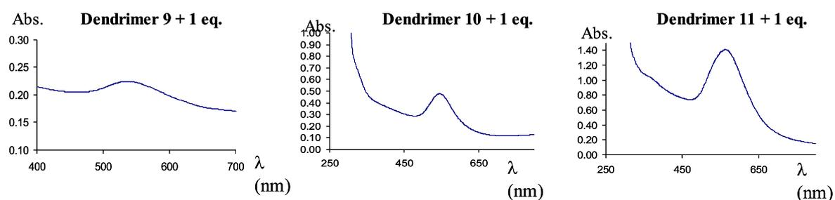
Figure 9. UV-vis spectra of AuNPs formed and stabilized by the dendrimers **9**, **10** and **11**.
