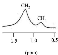
Fig. S1:  $^1\text{H}$  NMR spectrum of dodecanethiolate-AuNPs in  $\text{CDCl}_3$  ( $\delta$  ppm)
