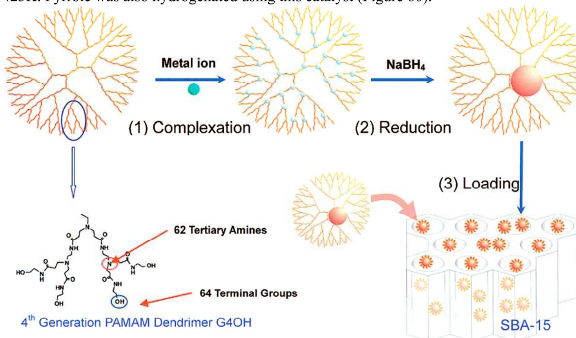
**Figure 60.** Synthesis of dendrimer encapsulated metal nanoparticles and the subsequent immobilization of the nanoparticle on mesoporous SBA-15 support. Reprinted with permission of the American Chemical Society (ref. 1043, Somorjai's group).
