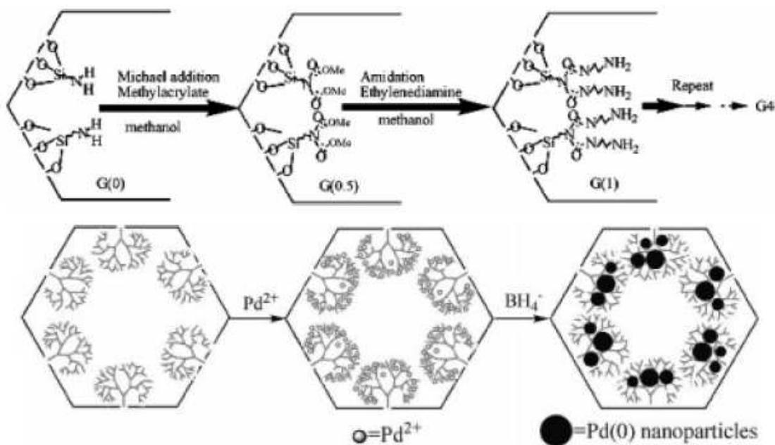
**Figure 43.** Preparation of SBA-15 supported dendrimers; formation of nanoparticles. Reprinted with permission of the American Chemical Society (ref. 858, Gao's group).
