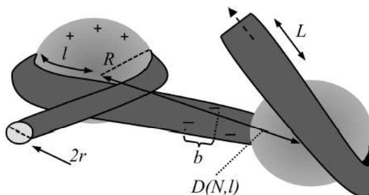
**Figure 84.** Proposed binding model between DNA of contour length  $L$ , radius  $r$ , and distance between negative charges  $b$  and G<sub>4</sub> PAMAM dendrimers modeled as hard spheres of radius  $R$ . The DNA is shown to wrap around the dendrimer with the length of the wrapping part equal to  $l$ , and a distance between the centers of two neighboring dendrimers,  $D(N, l)$ . Reprinted with permission of the American Chemical Society (ref. 1414, Qamhieh's group).
