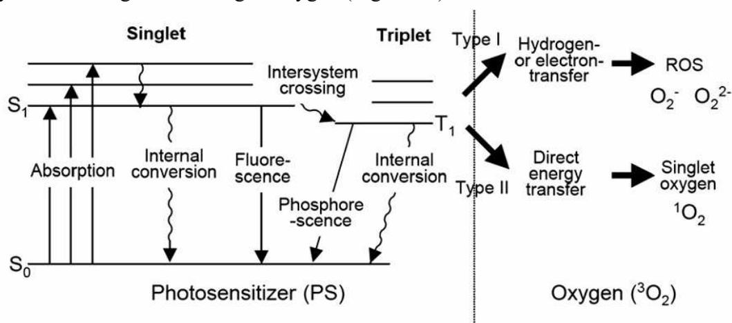
**Figure 89.** Jablonski diagram showing the energy transfer from photosensitizers (PSs) to molecular oxygen. Reprinted with permission of Elsevier (ref. 1487, Kataoka's group).
