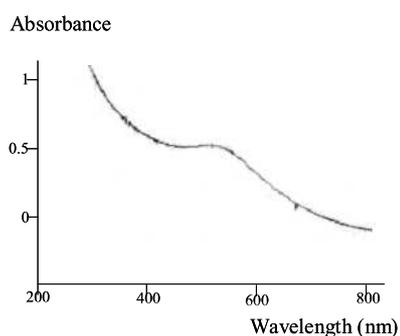
Fig. S13: UV-vis. spectrum of ferrocenyltriazolylkanethiolate AuNPs in CH<sub>2</sub>Cl<sub>2</sub>
