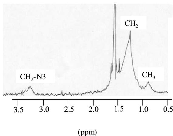
Fig. S6:  $^1\text{H}$  NMR spectrum of mixed dodecanethiolate-1-azidoundecanethiolate AuNPs in  $\text{CDCl}_3$  ( $\delta$  ppm)
