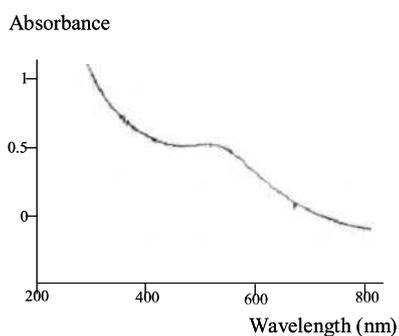
Fig. S20: UV-vis. spectrum of AuNPs with triallyl aryl dendron termini in  $\text{CH}_2\text{Cl}_2$
