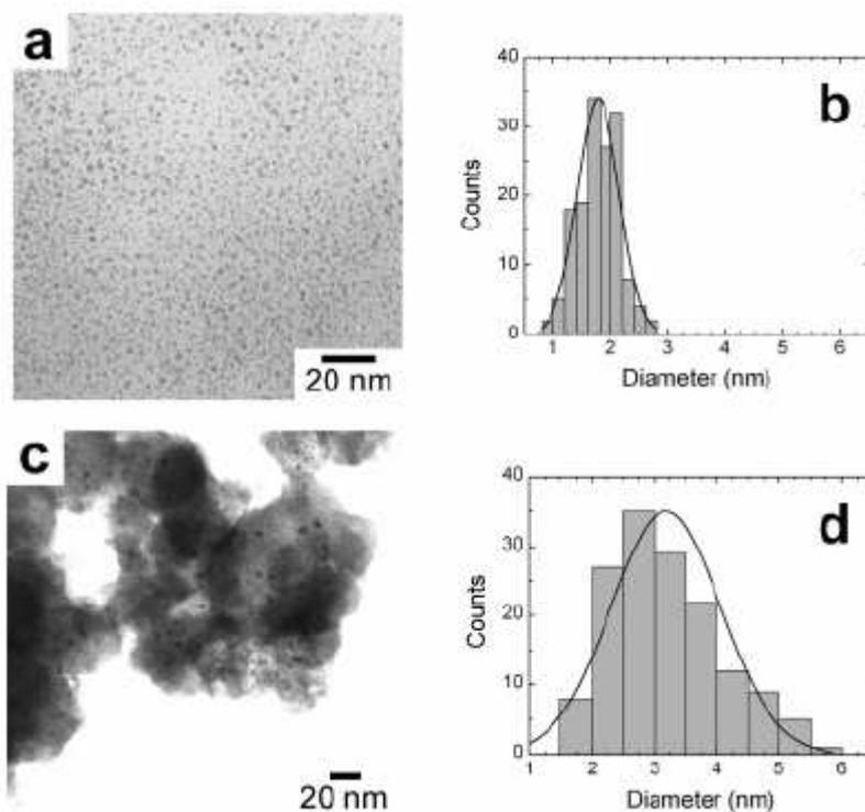
**Figure 58.** Bright-field TEM images and particle-size distributions for  $G_4\text{-NH}_2(\text{Pd}_{27.5}\text{Au}_{27.5})$  DENs prepared by co-complexation of the corresponding metal salts followed by reduction. (a), (b) As synthesized. (c), (d) After incorporation into the titania matrix and subsequent calcination at 500 °C under  $\text{O}_2$  and  $\text{H}_2$ . Reprinted with permission of the American Chemical Society (ref. 1011, Crooks's group).
