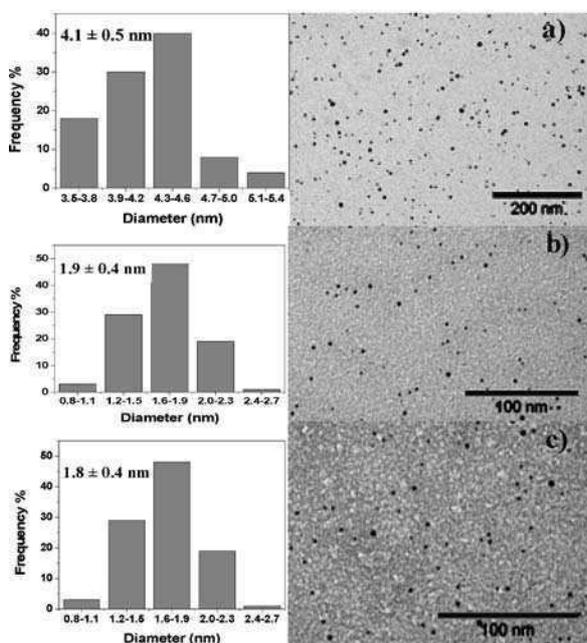
**Fig. 2** (a) Dendrimer  $G_0$ -27-TEG/AuNPs: TEM image and size distribution; (b) dendrimer  $G_1$ -81-TEG/AuNPs: TEM image and size distribution; (c) dendrimer  $G_2$ -243-TEG/AuNPs: TEM image and size distribution.
