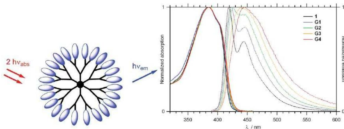
**Figure 13.** Schematic representation of dendrimeric two-photon absorbing fluorescent organic “nanodots”. Normalized absorption and emission spectra in toluene of dendrimers  $G_1$ – $G_4$  and model chromophore noted 1. Reprinted with permission of the Royal Society of Chemistry (ref. 276, Blanchard-Desce’s group).
