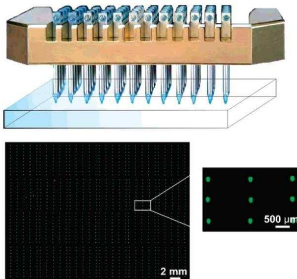
**Figure 39.** Robotic contact printing of DNA onto a flat dendri-stamp. Fragment of a fluorescence image of an aldehyde-terminated glass slide with an array of 400 spots of oligonucleotide labeled with fluorescein printed using a dendri-stamp. Reprinted with permission of the American Chemical Society (ref. 716, Reinhoudt's group).
