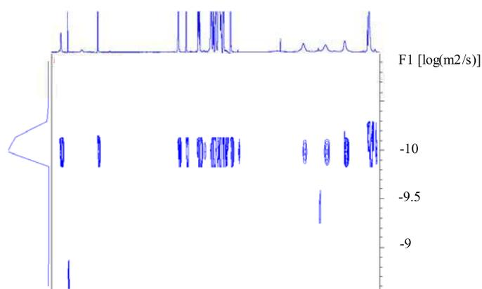
Figure 3. DOSY spectrum of the dendrimer **4**.  $D = 1.16 (\pm 0.1) \times 10^{-10} \text{ m}^2/\text{s}$ ,  $R_h = 4.9 (\pm 0.1) \text{ nm}$ ; ( $D$ : diffusion coefficient;  $R_h$ : hydrodynamic radius).
