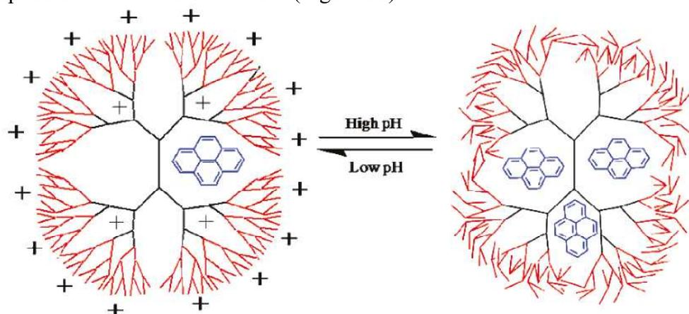
**Figure 33.** Schematic representation of pyrene encapsulation in PPI-core:PAMAM-shell dendrimers at acidic and basic *pH*. Reprinted with permission of the American Chemical Society (ref. 567, Imae's group).
