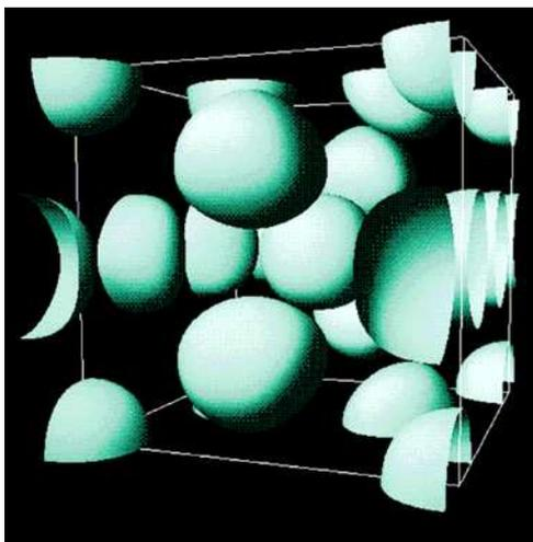
**Figure 3.** The 3D electron density distribution of the  $Pm\bar{3}n$  Cub phase ( $a = 79.2 \text{ \AA}$  at  $80^\circ\text{C}$ ) of the spherical supramolecular dendrimers self-assembled from 16 monodendrons. These isoelectron surfaces were generated from XRD by Fourier synthesis with the structure factor phases determined by TEM. Reprinted with permission of the American Association for the Advancement of Science (ref. 89, Hudson's group).
