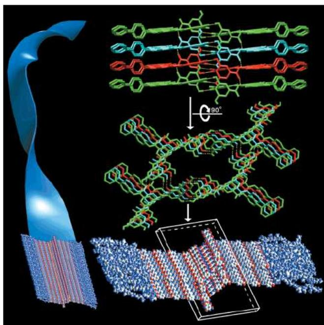
**Figure 6.** Side view of the ribbonlike structure taken directly from the crystal structure of a dendrimer shows color-coded hydrogen-bonded tetramers (upper right) stacked on top of each other along the direction of the crystal (top view is shown in the middle right). Schematic (left and bottom right) representation of the proposed structure for a DRC nanoribbon. Reprinted with permission of the American Chemical Society (ref. 124, Stupp's group).
