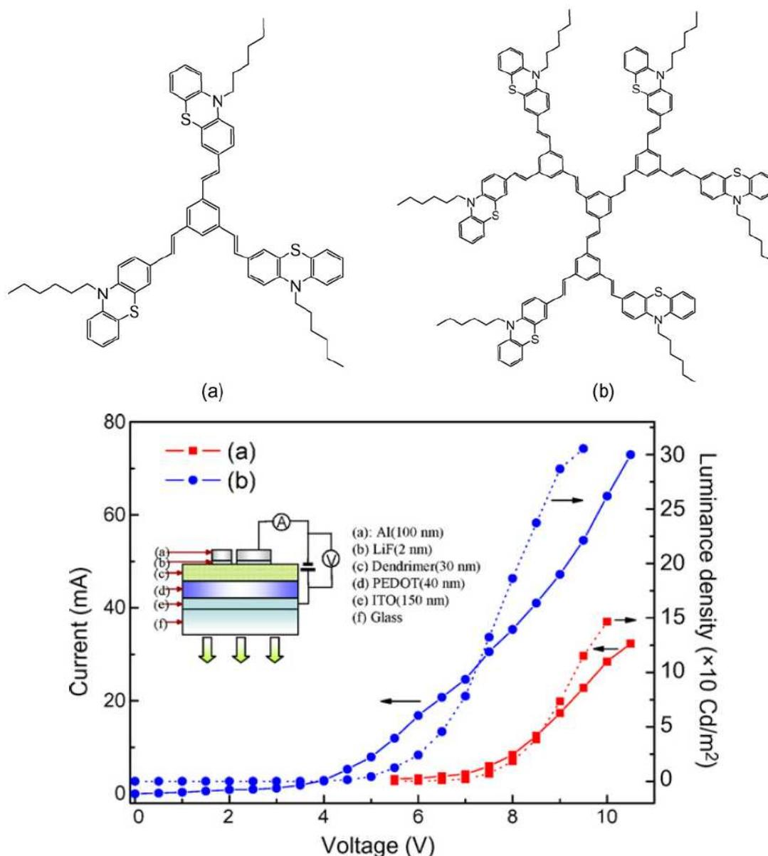
**Figure 19.** Current–voltage–luminance curves for two LEDs made of dendrimers. Reprinted with permission of Elsevier (ref. 397, Choi’s group).
