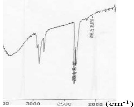
Fig. S12: IR spectrum of ferrocenyltriazolylkanethiolate AuNPs
