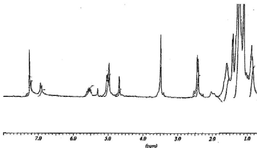
Fig. S18:  $^1\text{H}$  NMR spectrum of AuNPs with triallyl aryl dendron termini in  $\text{CDCl}_3$  ( $\delta$  ppm)
