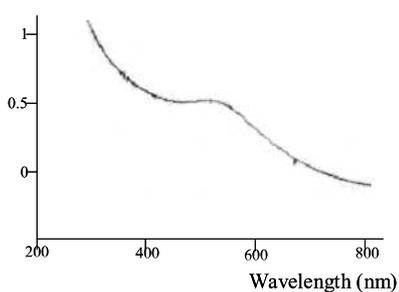
Fig. S17: UV-vis. spectrum of AuNPs with tetraethyleneglycol termini in  $\text{CH}_2\text{Cl}_2$
