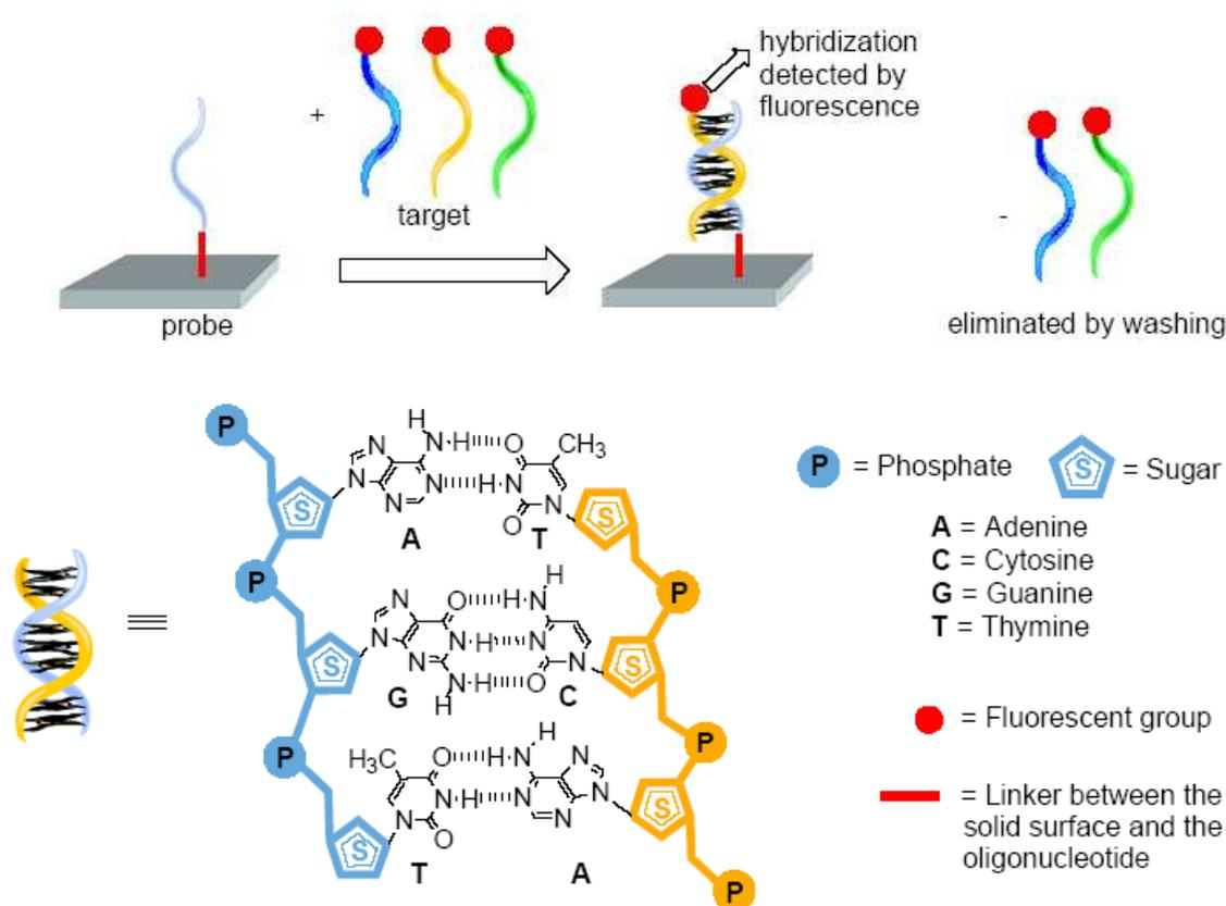
**Figure 102.** Principle of a DNA chip or DNA array. Only the oligonucleotide complementary to the one immobilized on the surface can hybridize. The hybridization occurs through supramolecular recognition of complementary bases (Adenine with Thymine, and Cytosine with Guanine) linked to the sugar and phosphate backbones, as illustrated by one example. Reprinted with permission of the Molecular Diversity Preservation International (ref. 1598, Majoral's group).
