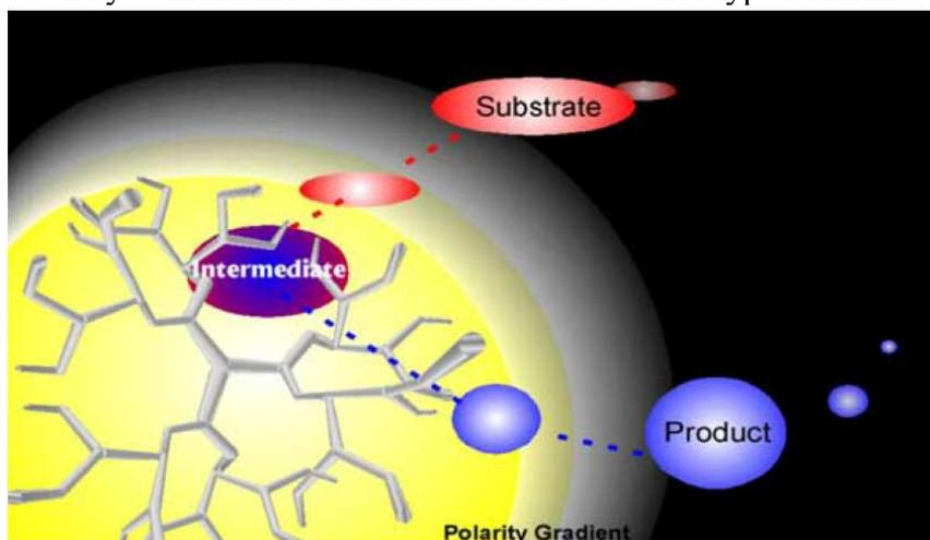
**Figure 53.** Illustration of substrate migration into the dendrimer interior. The nanoenvironment is greatly influenced by the branching units and creates a gradient of polarity with respect to the distinct interior and exterior solvent. These favorable conditions encourage substrate concentration and transition state stabilization. The resulting product is released from the nanoreactor into the solvent. Reprinted with permission of Elsevier (ref. 971, Fréchet’s group).
