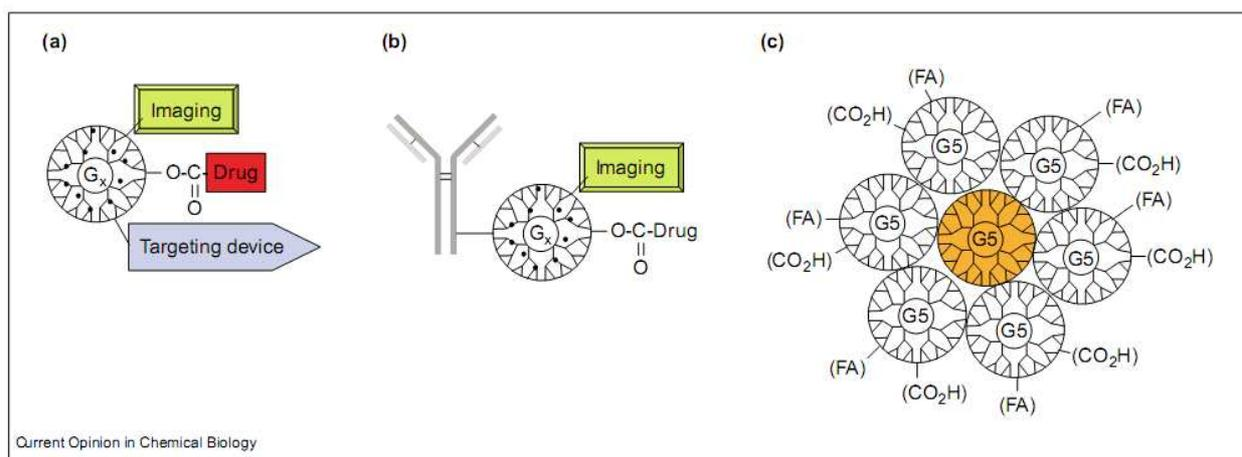
**Figure 62.** Dendritic nanodevices for therapeutic applications. (a) Surface-modified PAMAM dendrimer for targeting, imaging and drug delivery. (b) Antibody–dendrimer conjugate. (c) Tecto(dendrimer). FA, folate. Reprinted with permission of Elsevier (ref. 1088, Baker Jr.’s group).
