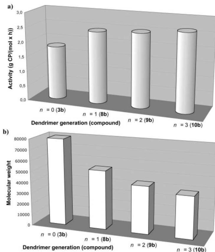
**Figure 48.** (a) Activities for  $G_n$ -ONNMe<sub>2</sub>[Pd(MeCN)Me<sup>+</sup>] and (b) copolymer Mw values obtained using neat TBS as a solvent. Reprinted with permission of the American Chemical Society (ref. 905, Flores's group).
