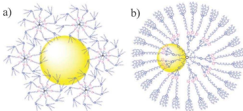
**Fig. 1** (a) AuNPs stabilized by several  $G_0$  dendrimers; (b)  $G_1$ -dendrimer-encapsulated AuNPs. Reprinted with permission of the Royal Society of Chemistry (ref. 24, Astruc's group).
