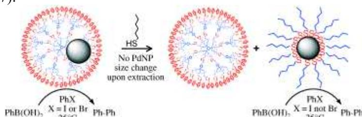
**Figure 56.** Extraction of PdNPs from DSNs or DENs with hexanethiol without any change in the size of the PdNPs to produce air- and water-stable, catalytically active hexanethiolate PdNPs. Reprinted with permission of Wiley-VCH (ref. 1002, Astruc's group).
