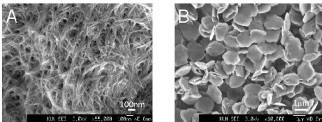
**Figure 5.** The nanoscale morphology observed using SEM for the two-component gelation system. a = 2 : 1 dendron:diamine ratio. b = 1 : 4.5 dendron:diamine ratio. Reprinted with permission of the American Chemical Society (ref.108, Smith's group).
