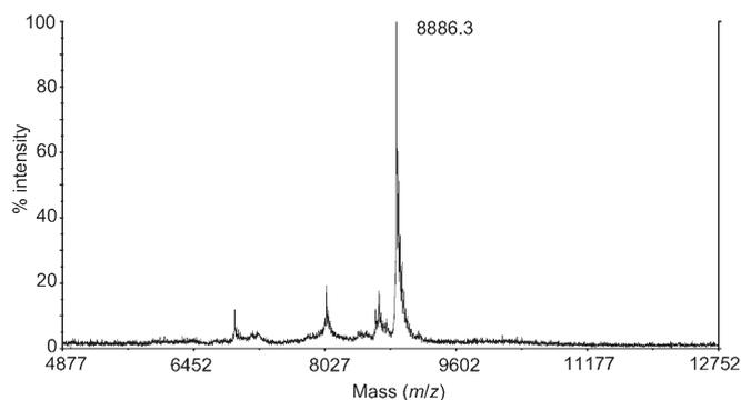
Figure 1. MALDI-TOF mass spectrum of G<sub>1</sub> dendri-27-benzoic acid **8**.
