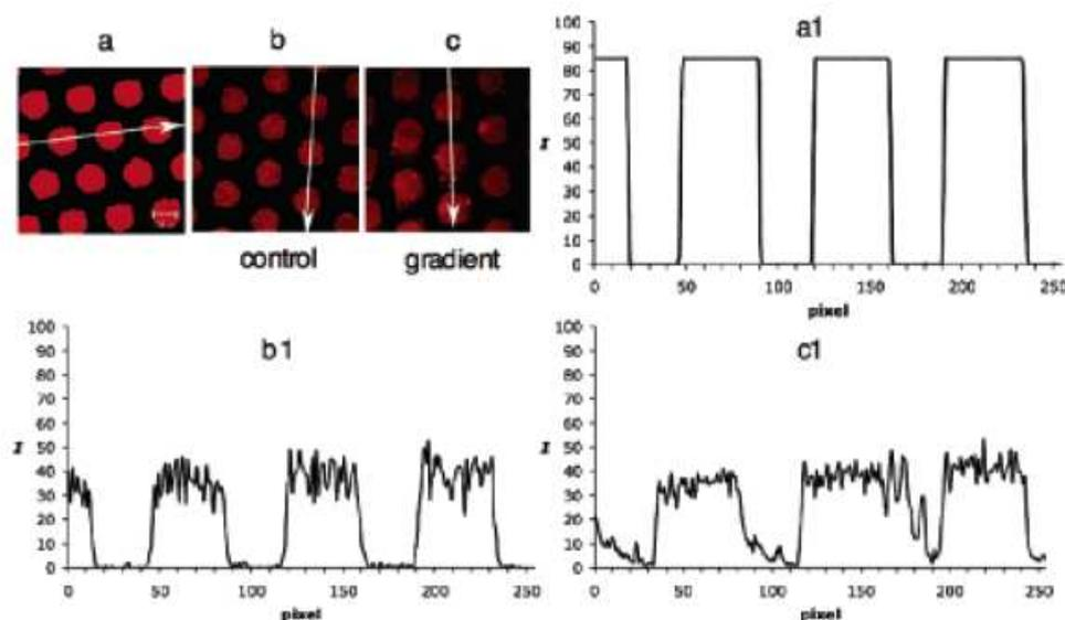
**Figure 8.** Averaged fluorescence profiles and their corresponding confocal microscope images of dendrimers (a) before immersion and (b) control and (c) gradient substrates, after 16h of immersion. Reprinted with permission of the American Chemical Society (ref. 157, Reinhoudt's group).
