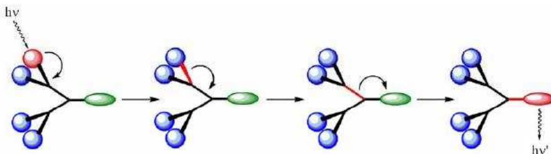
**Figure 10.** Schematic illustration of a dendrimer as an antenna. The excitation energy  $h\nu$  (shown in red) migrates along the dendrimeric framework until it reaches the core where the energy is used for some purpose such as a chemical reaction. Reprinted with permission of Elsevier (ref. 210, Flomembom's group).
