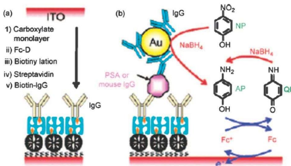
**Fig. 14** (a) Schematic representation of the preparation of an immunosensing layer. (b) Schematic view of electrochemical detection of mouse IgG or prostate specific antigen. Reprinted with permission of the American Chemical Society (ref. 85, Wang's group).
