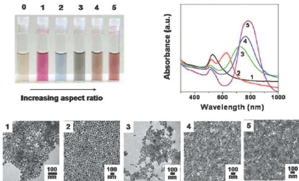
**Fig. 2** The optical properties of gold and silver nanoparticles change drastically with nanoparticle shape. The photograph shows aqueous solutions of 4 nm gold nanospheres (vial 0) and progressively higher aspect ratio gold nanorods (1–5). The optical spectra and transmission electron micrographs for the particles in vials 1–5 are also shown. Scale bars in micrographs are all 100 nm. Reprinted with permission of the Royal Society of Chemistry (ref. 26, Murphy's group).
