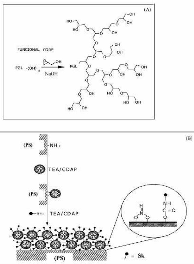
**Figure 74.** (A) Schematic diagram of the PGLD synthesis and (B) immobilization of the bioconjugate PGLD-Sk onto wells of ELISA (PS) plates. The epifluorescence microscopy results indicate that PGLD-Sk coating showed an improved antithrombogenic character relative to the uncoated ELISA plates. Reprinted with permission of Springer Science (ref. 1212, Roman's group).
