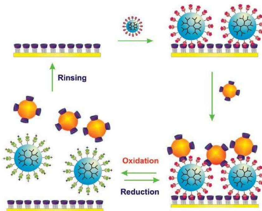
**Figure 38.** Illustration of the adsorption and desorption of  $\beta$ -CD-functionalized NPs onto and from  $\beta$ -CD SAMs with Fc dendrimers as a reversible supramolecular glue. Reprinted with permission of the American Chemical Society (ref. 714, Huskens's group).
