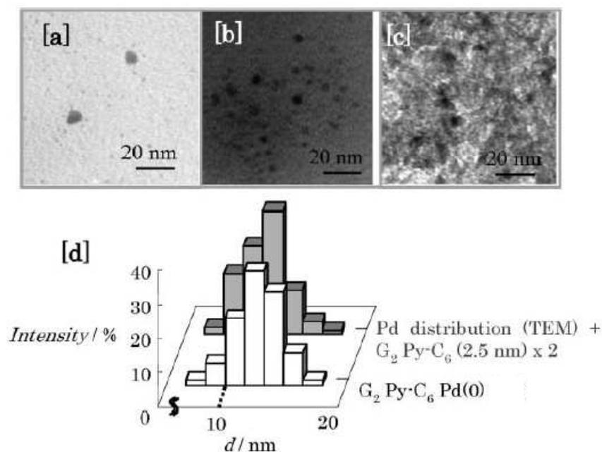
**Figure 54.** TEM images of Pd nanoparticles encapsulated within the G<sub>2</sub> dendrons; (a) G<sub>2</sub> Py-CO<sub>2</sub>Me Pd(0), (b) G<sub>2</sub> Py-C<sub>6</sub> Pd(0), (c) G<sub>2</sub> Py-C<sub>12</sub> Pd(0) and (d) the size distributions of G<sub>2</sub> Py-C<sub>6</sub> Pd(0). Reprinted with permission of the Royal Society of Chemistry (ref. 990, Kaneda's group).
