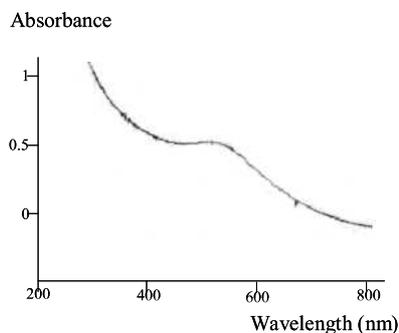
Fig. S3: UV-vis. Spectrum of dodecanethiolate-AuNPs in  $\text{CH}_2\text{Cl}_2$
