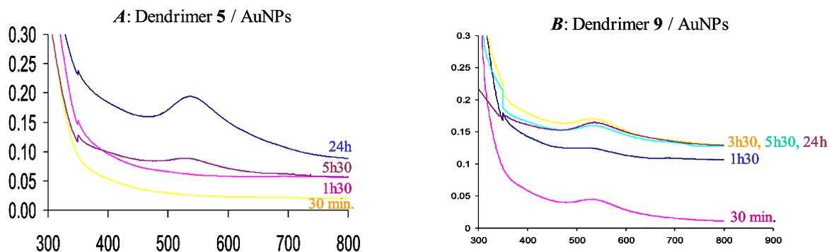
Figure 8. UV-vis spectra of AuNPs formed and stabilized by the dendrimers **5** and **9** at different times.
